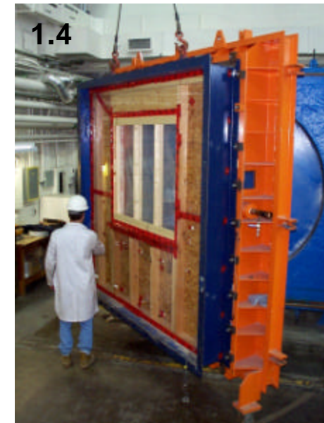
Figure 1.3 - Inside view of apparatus showing test specimen (sizes up to 2.44 by 2.44-m). The exterior cladding faces the inside of the apparatus.
