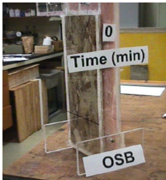
Figure B.45 - Set-up for test case No. 2 with OSB backing
