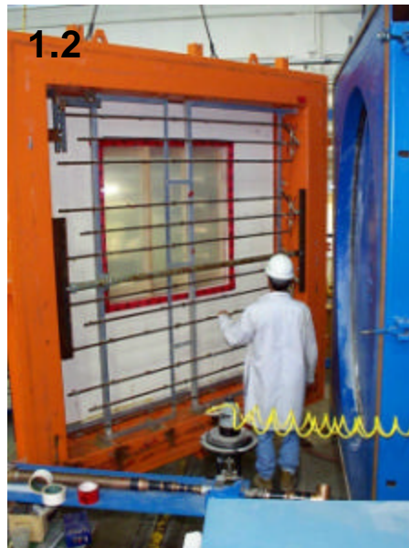
Figure 1.3 - Inside view of apparatus showing test specimen (sizes up to 2.44 by 2.44-m). The exterior cladding faces the inside of the apparatus.
