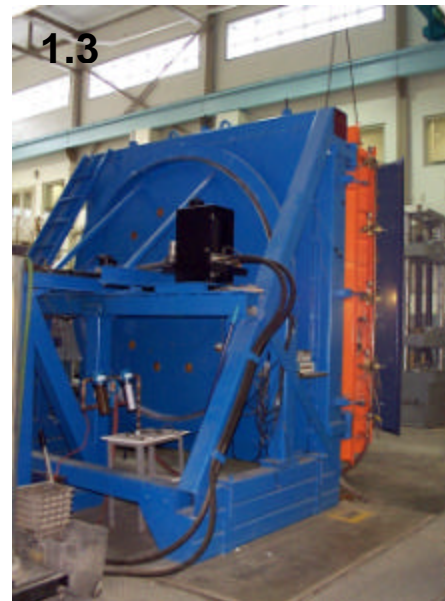
Figure 1.3 - Inside view of apparatus showing test specimen (sizes up to 2.44 by 2.44-m). The exterior cladding faces the inside of the apparatus.
