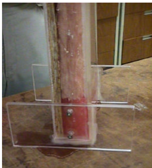
Figure B.47 - Test case No. 2 a few minutes after water entry
