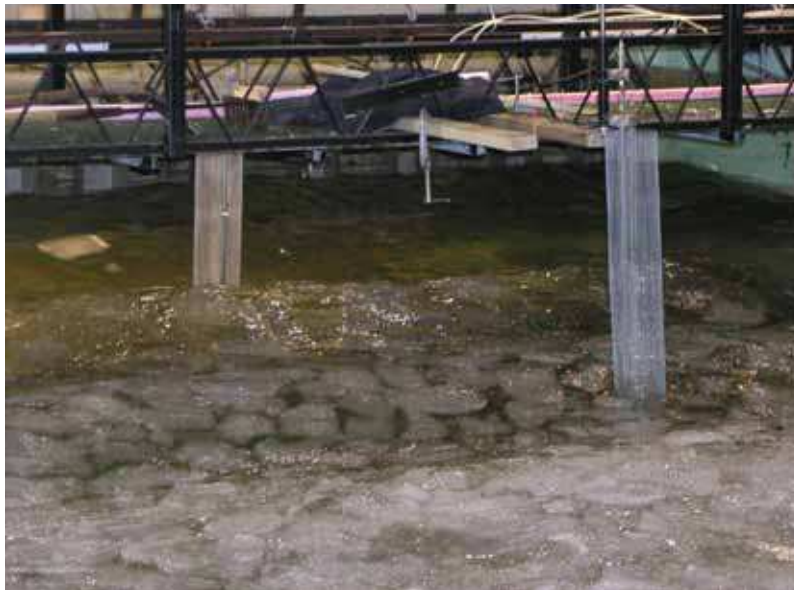
Figure 8 Set-up of wave probes spanning service carriage.
