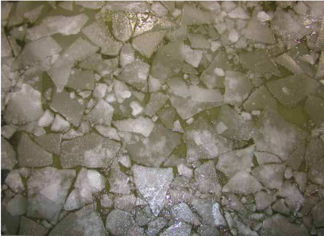
Figure 3 Piece size distribution after breaking up an ice sheet.
