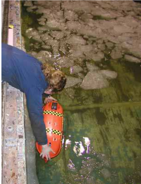
Recovery of TEMPSC at side of ice tank
