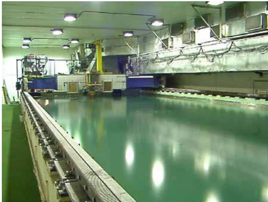
Figure 1 Ice tank at the Canadian Hydraulics Centre.
