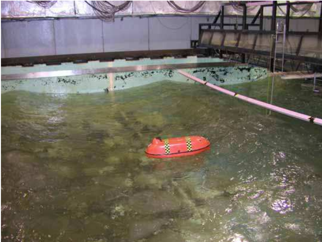
TEMPSC in 5/10ths ice concentration, 25 mm ice thickness, swell wave conditions
