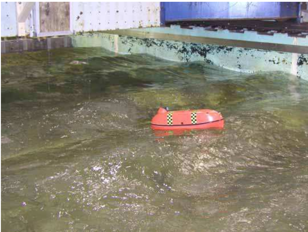
TEMPSC in 5/10ths ice concentration, 25 mm ice thickness, storm wave conditions
