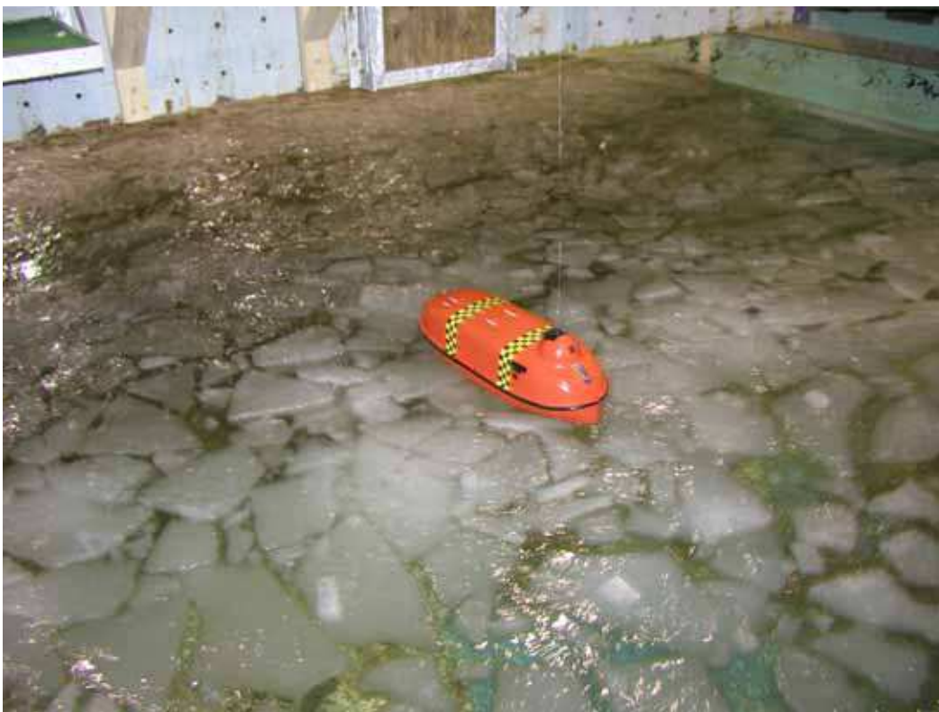
Test deployment in 8/10ths ice concentration, 50 mm ice thickness
