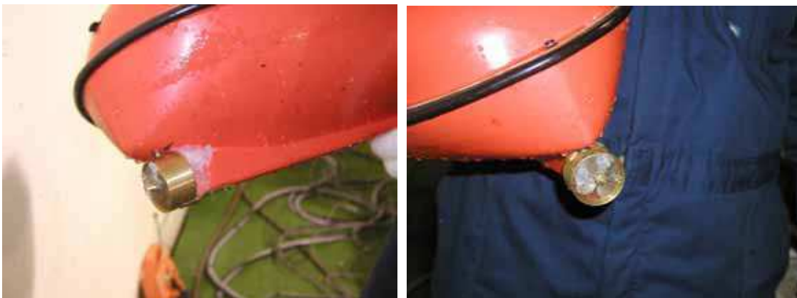
Figure 19 Photographs showing ice lodged in the propeller after some tests.
