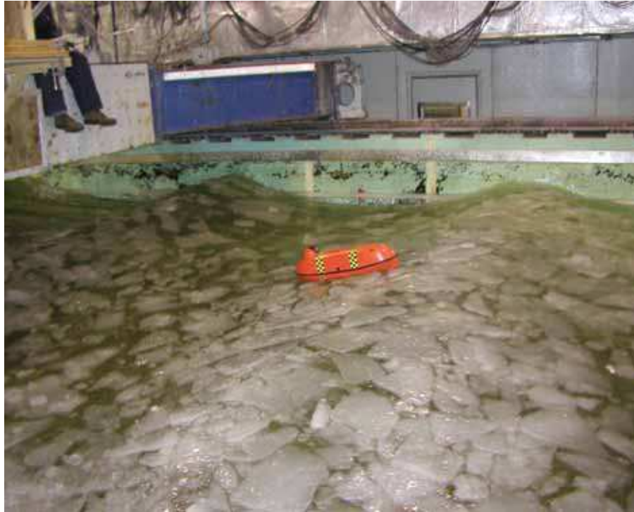
Figure 12 Photograph taken from the side of the tank of TEMPSC traveling through swell waves.
