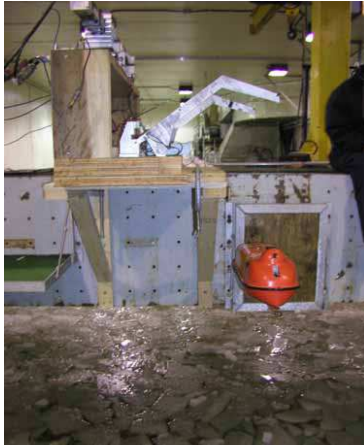
Figure 5 TEMPSC model with launching system
