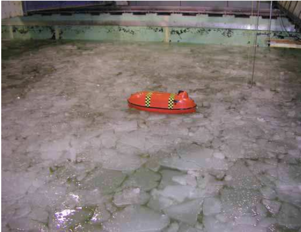
Figure 14 Photograph during a test, showing the rafting and dense concentration of ice at the end of the tank.
