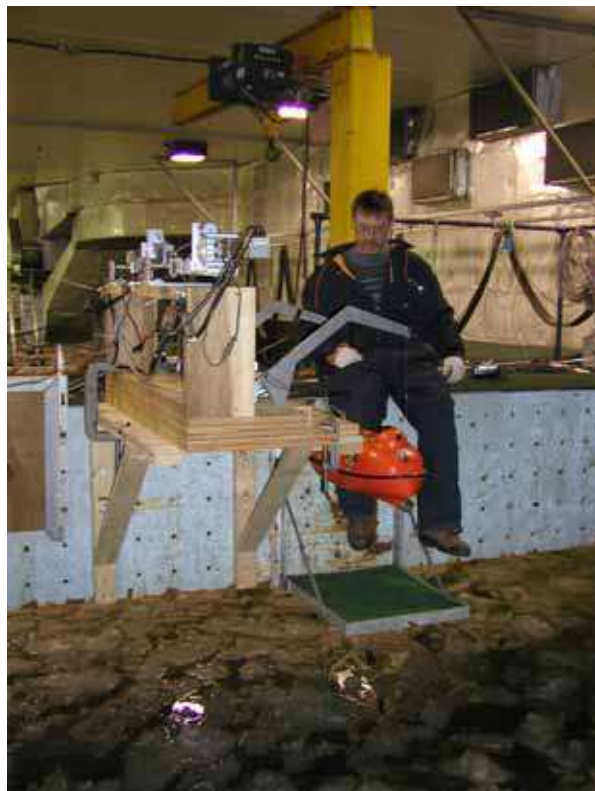
Returning TEMPSC to initial deployment position on davit system
