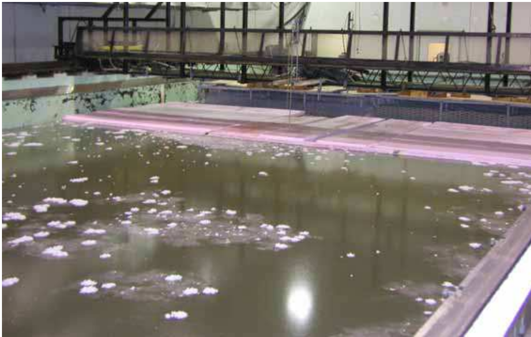
Figure 2 Preparing an ice sheet. Rigid insulation covers the water surface in order to control the concentration of ice in the tank.
