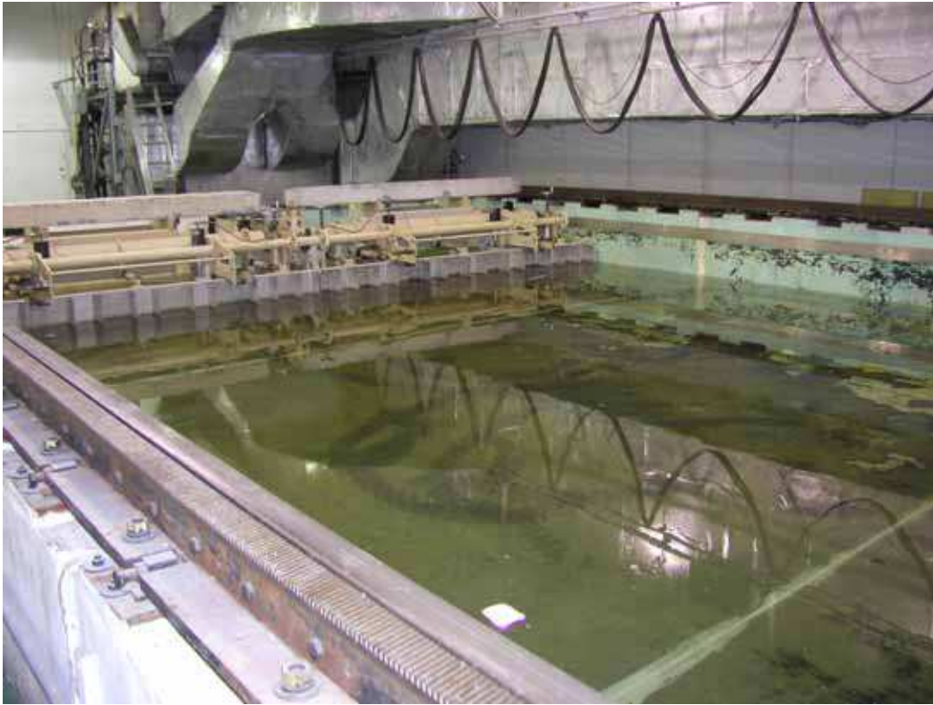
Ice tank with wave machines
