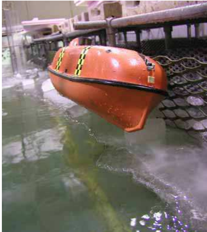
Figure 18 TEMPSC beached on ice ledge attached to wave absorbers.
