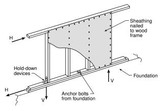
*Figure 1. Simplified diagram of main seismic forces acting on a shear wall*
