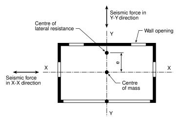
Figure 3. Schematic of an unsymmetrical building layout. Seismic forces in X-X direction cause twisting action in horizontal plane due to eccentricity "e," the distance between the centre of storey mass and the centre of storey shear wall resistance.
