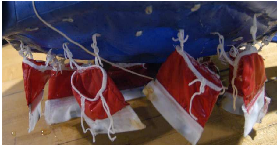
Figure 3.4: Stability pockets attached to model IOT 721.
