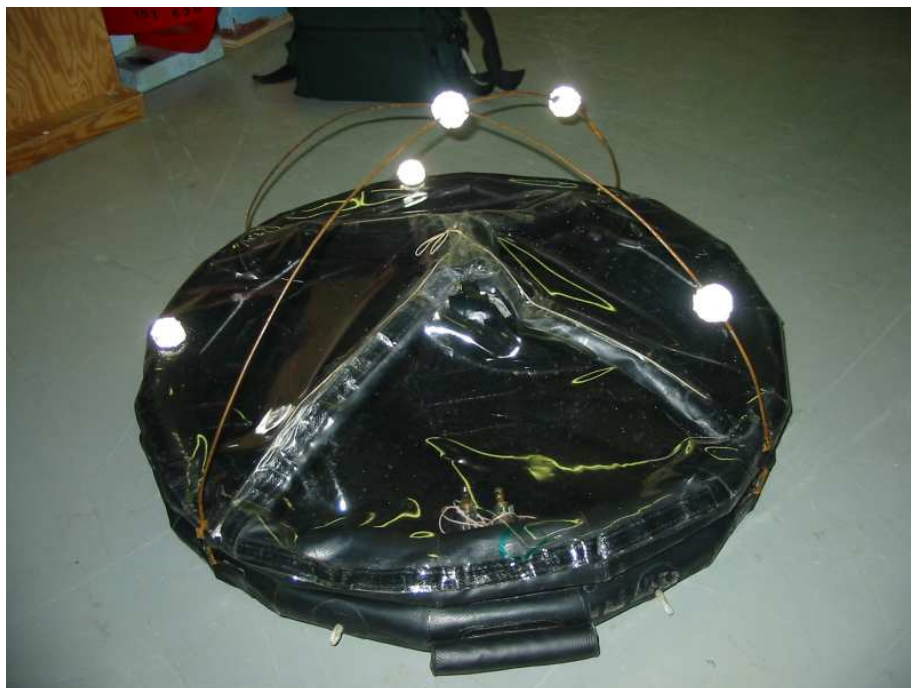
Figure 3.2: Model IOT 721 of a 16-person life raft with wire frame and Qualysis optical tracking markers attached.
