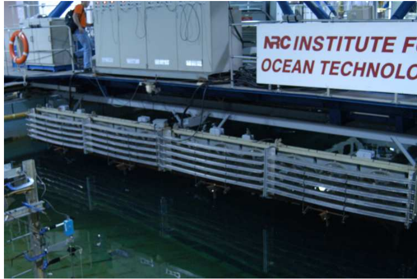
Figure 3.6: Wind fans mounted on the bottom of the main tow carriage.
