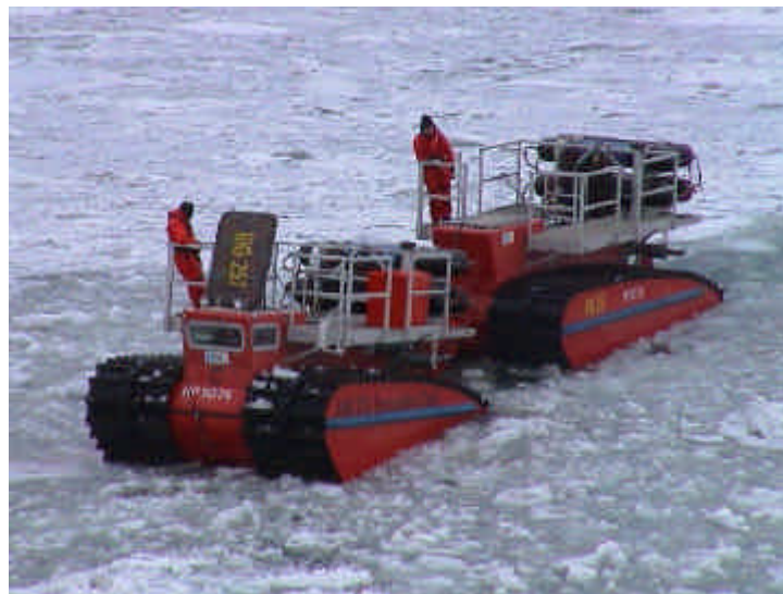
Figure 5.21: Relatively thin ice conditions in which an ARKTOS craft has considerable difficulty in making any significant forward progress. In this photo, it is “wallowing” at a very low speed of advance.
