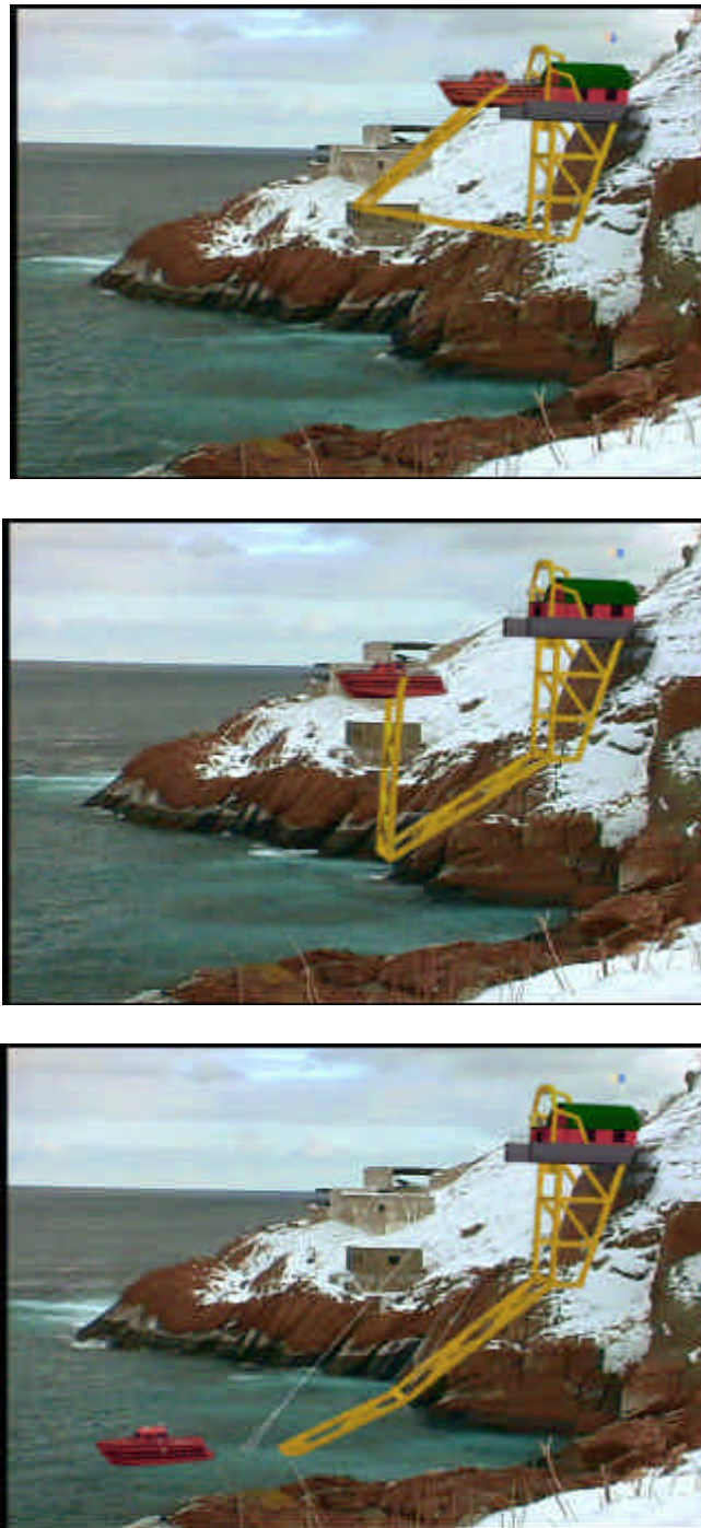
Figure 4.8: Views of the Seascope articulated launching arm, which is lowered on a winch and deploys a yoke mounted TEMPSC unit “out and away” from a platform.
