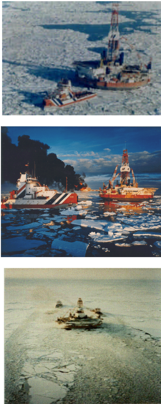
Figure 5.10: Representative views of the Kulluk in heavy pack ice conditions during summer ice intrusions (upper), in partial ice coverage situations (middle), and in thin freeze-up situations, including the type of managed ice floes typically seen around the platform.
