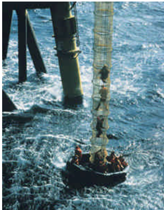
Figure 4.12: An illustration of the MES escape chute system, with people moving down it during a training exercise in a calm open water situation.
