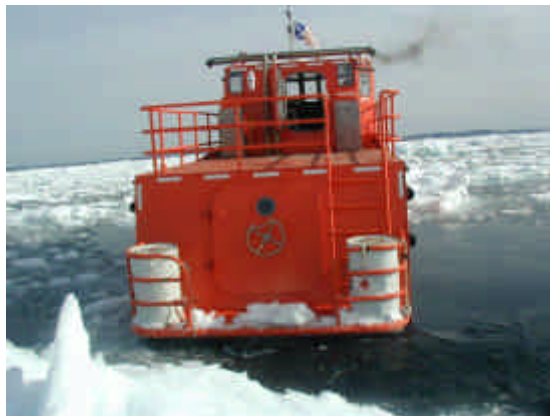
Figure 4.9: Views of the Seascope prototype TEMPSC unit, taken at dockside (upper) and during trials in late spring ice conditions off Newfoundland (lower two photos).
