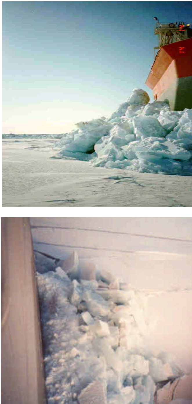
Figure 5.8: Representative views of the type of ice interaction behaviours that were seen immediately adjacent to the Molikpaq in moving pack ice conditions.
