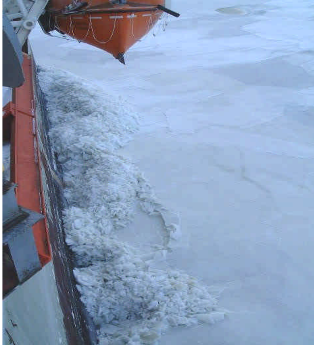
Figure 4.3: The hull of a typical TEMPSC lifeboat, in this case, one of 50 man units installed in standard davits on the Molikpaq caisson. Lowering the craft into the failing ice zone present at the time of this photo would crush it
