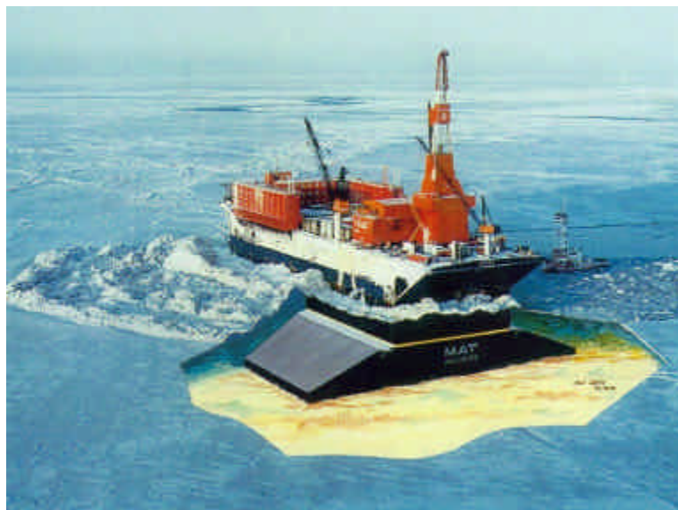
Figure 5.5: Representative views of thin pack ice around the SSDC during the freeze-up period, and the type of ice rubble and downdrift wakes often seen adjacent to it. The lower photo, taken during late freeze-up, shows a cut-away of the MAT base used during later SSDC deployments in the Alaskan Beaufort Sea, in its landfast ice zone.
