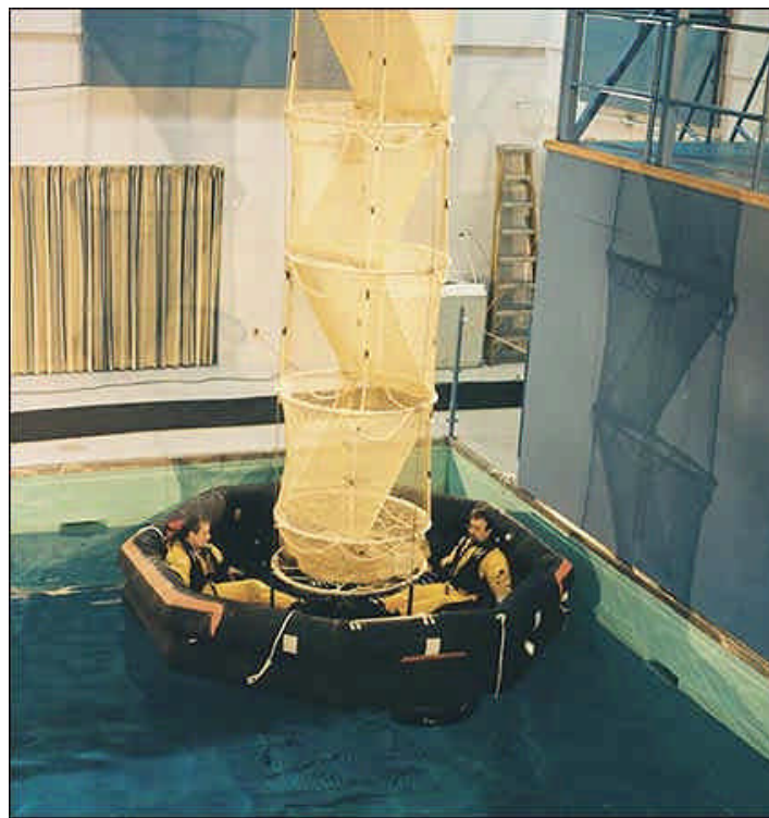
Figure 4.11: A view of the Skyscape system being employed during personnel training exercises in “calm open water conditions”.
