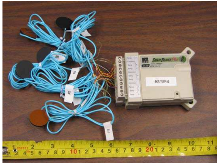
Figure 4.2: Self contained data loggers connected to heat flow sensors (second logger is magnetically attached behind logger “Skin Temp A2” pictured in photo.)
