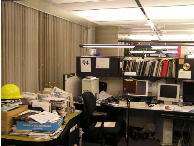
Figure 7. View from workstation A to towards workstation C in office 8B1 showing the small side panel blocking reflections of the adjacent windows.
