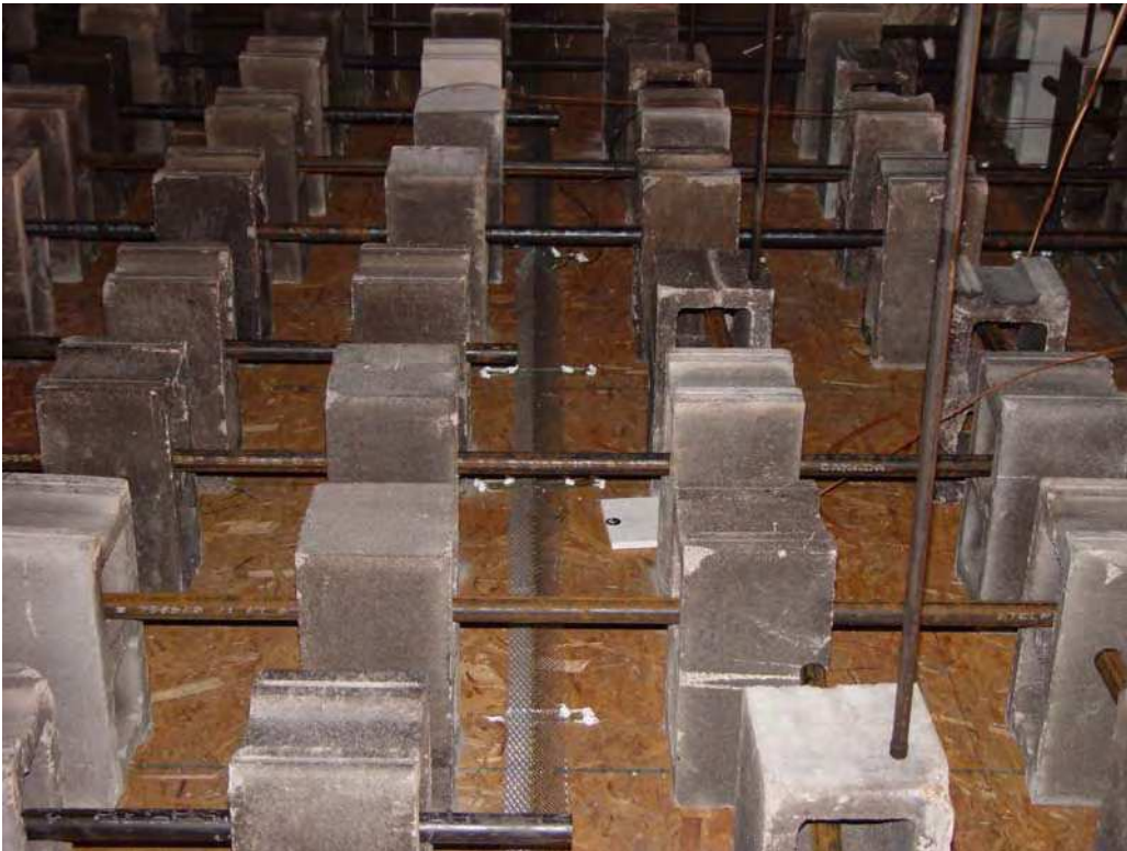
Figure 19. Device to hold the loading blocks
