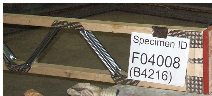
Figure 3: Steel web wood trusses with 65 x 40 mm wood flanges.
