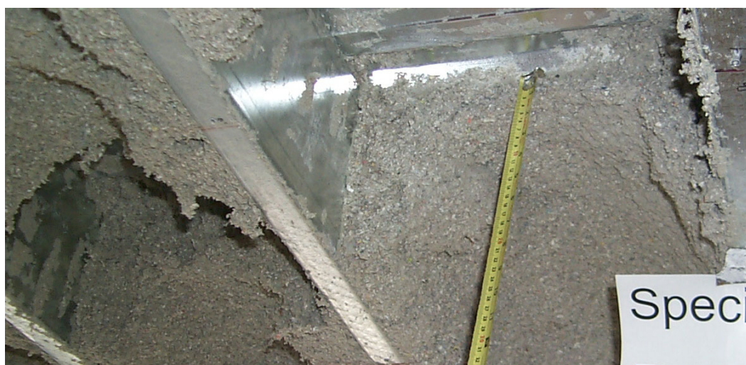
Figure 5: Sprayed-on cellulose applied to steel C-joist floor.
