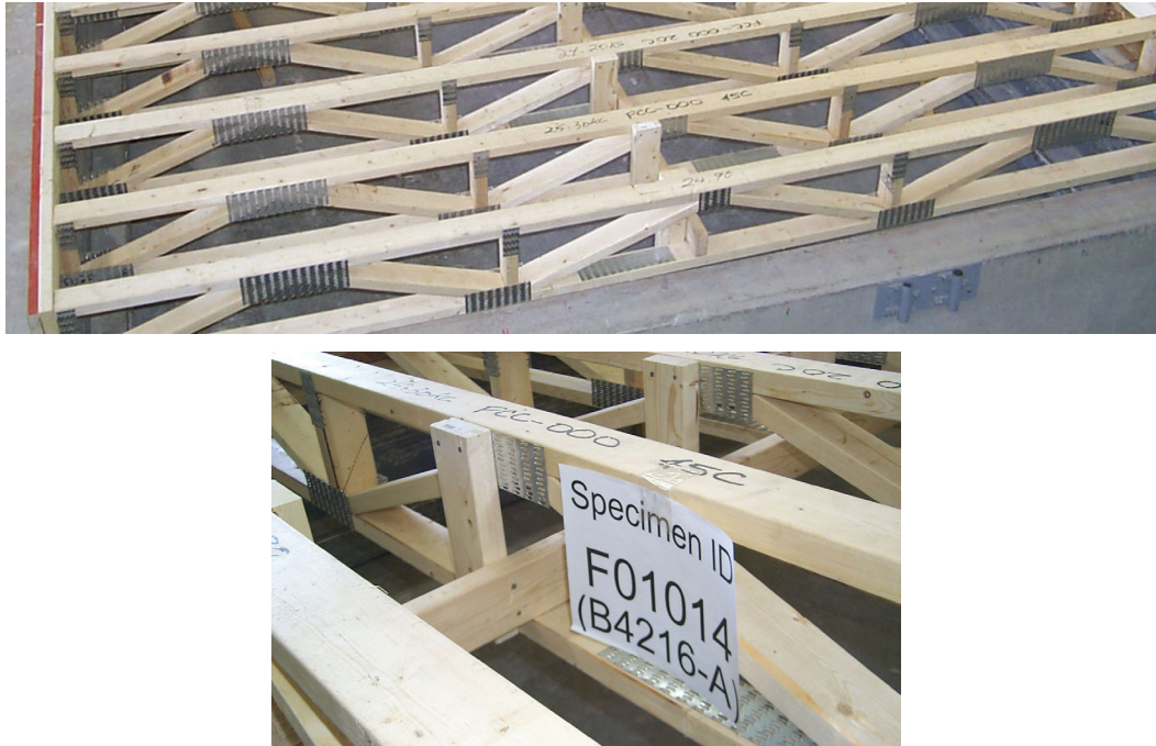
Figure 2: Metal-plate-connected wood truss framework. The trusses were formed from 38 x 89 mm lumber. The truss depth was 305 mm.
