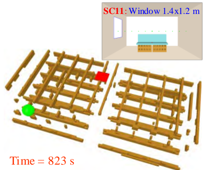
Figure 3-4 Status of the wood cribs when the burning stopped in SC1, SC3 & SC11 (HRR = ~1 kW) and at the end of simulation in SC10 (HRR ~ 1500 kW at 900 s)
