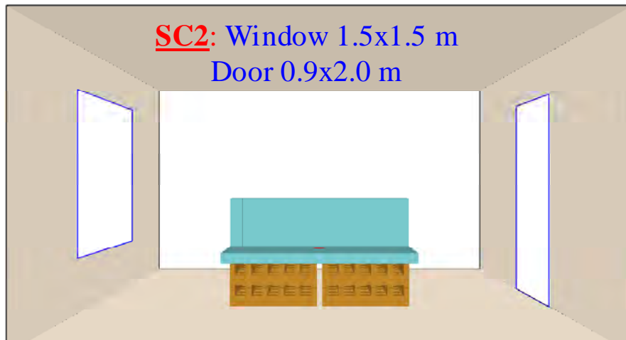
Figure 1-3 Ventilation parameters for scenarios using a window opening (different sizes) and doorway (same size) facing each other
