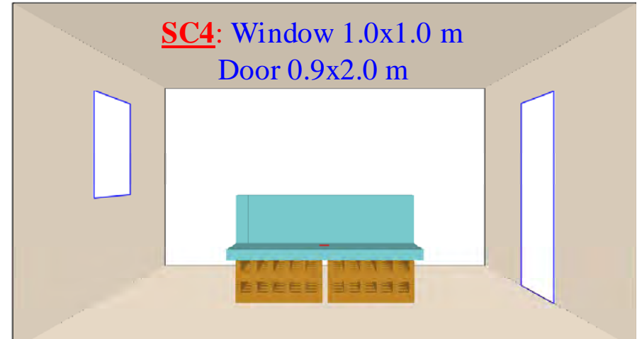
Figure 1-3 Ventilation parameters for scenarios using a window opening (different sizes) and doorway (same size) facing each other
