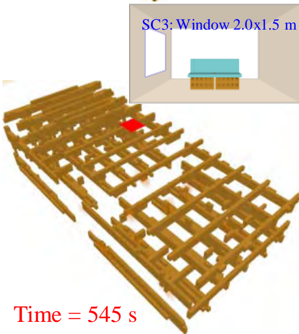
Figure 3-4 Status of the wood cribs when the burning stopped in SC1, SC3 & SC11 (HRR = ~1 kW) and at the end of simulation in SC10 (HRR ~ 1500 kW at 900 s)
