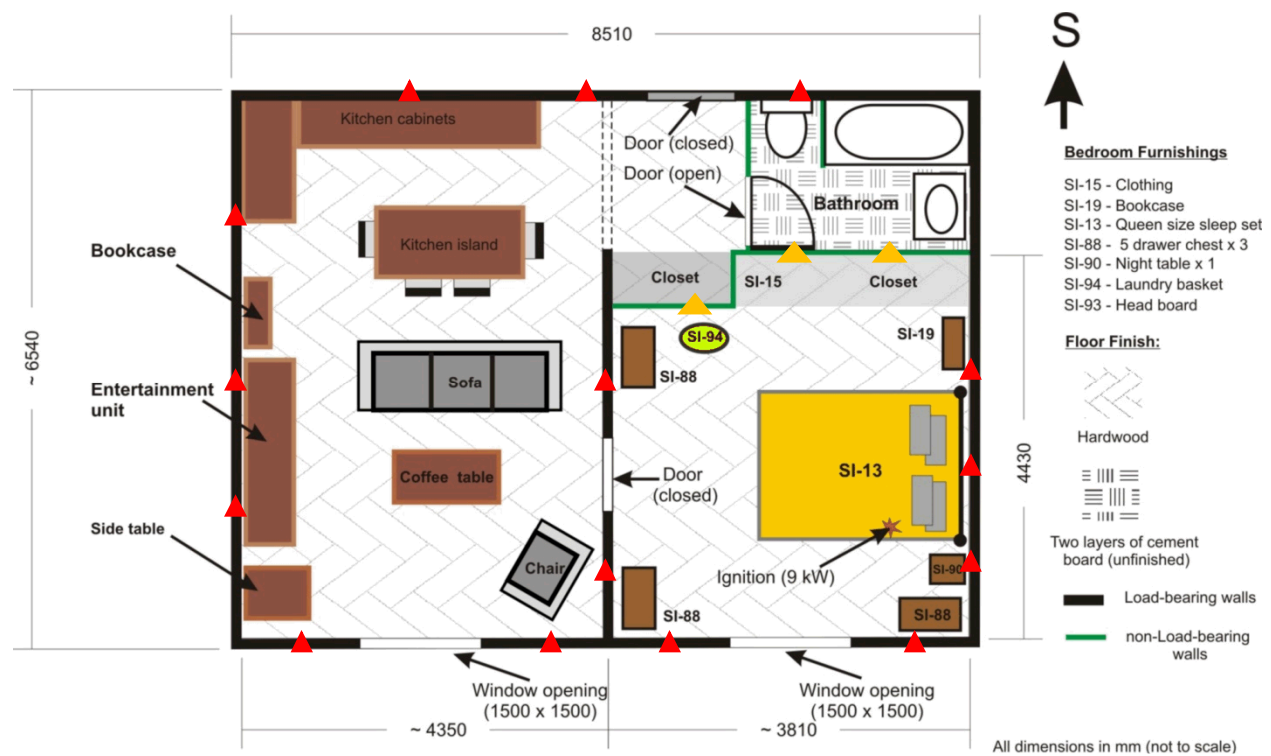
Figure 8. Sketch showing locations of thermocouples in wall cavities. (The locations indicated by ▲ had thermocouples located at the 0.6, 1.2 and 1.8 m heights. The locations indicated by ▲ had a single thermocouple at the 1.8 m height.)
