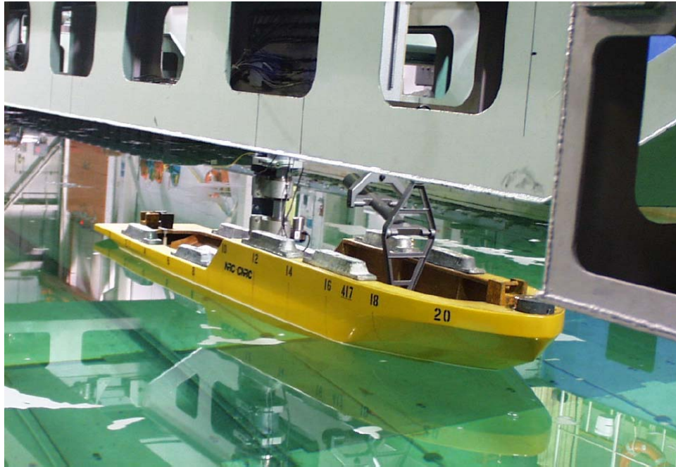
Figure 1a: Tow Post Test Setup.
