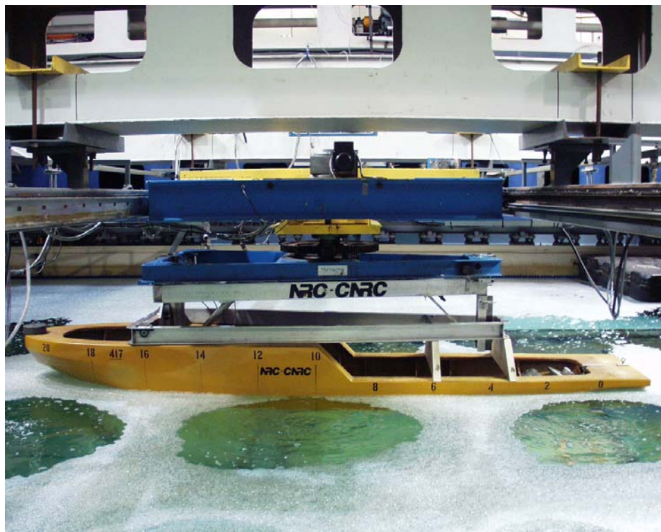
Figure 1b: Planar Motion Mechanism (PMM) Test Setup.
