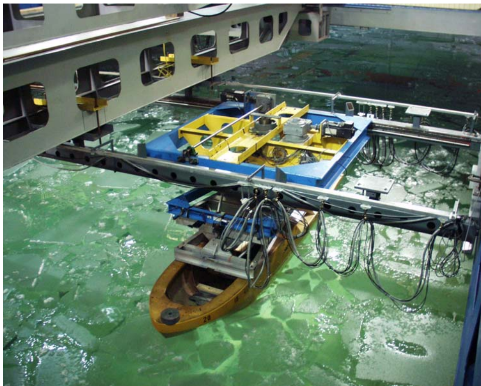
Figure 5b: Typical test run in broken ice (Phase III).
