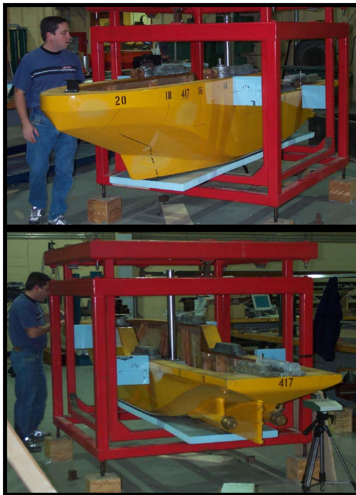
Figure 2b: Terry Fox Model on the swing frame on the Shop Floor.
