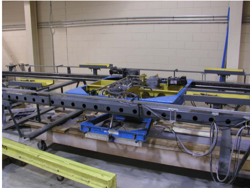
Figure 3a: Actual Planar Motion Mechanism on the Shop Floor.
