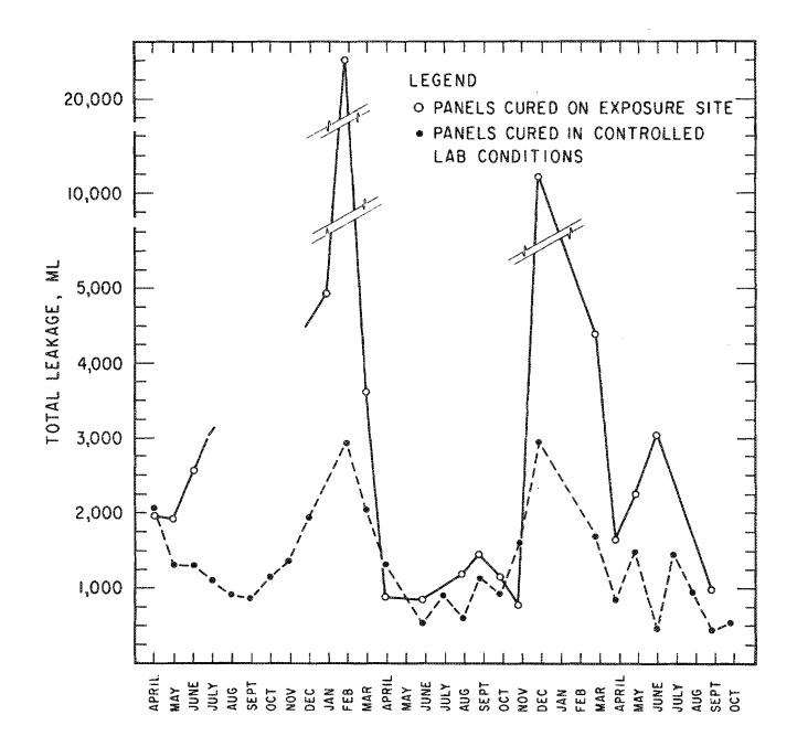
FIGURE 2 LEAKAGE TOTALS FOR LIME-MORTAR PANELS
