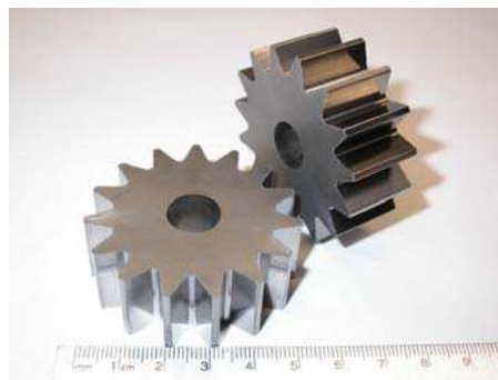
Figure 3. Sprockets produced in this study (2" O.D., 0.75" Height, 7.0\text{ g/cm}^3 )
