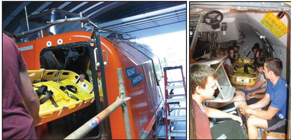
Figure 4.1: A Stoke's Litter being loaded into a 50-person TEMPSC (left), and the stretcher once placed inside a fully loaded lifeboat (right).
