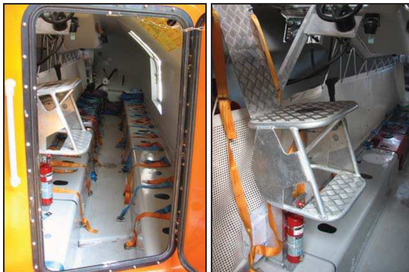
Figure 2.4: A view of the starboard TEMPSC bench seats from the stern hatch (left), and the coxswain's chair (right). The bulkhead created using blue and purple sandbags can be seen at the far end of the bench seats.
