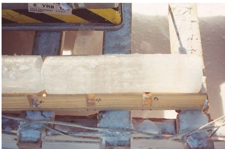
Figure 3 Fragments of ice core used for property measurements
