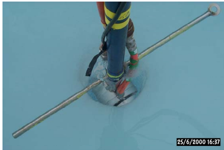
Figure 4 Borehole jack indenter inserted in ice borehole (courtesy of D. Bradley)
