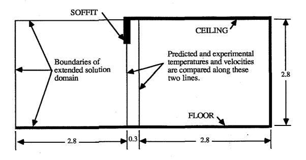
Figure 4: Solution domain and locations where temperature and velocities are computed for model validation.
