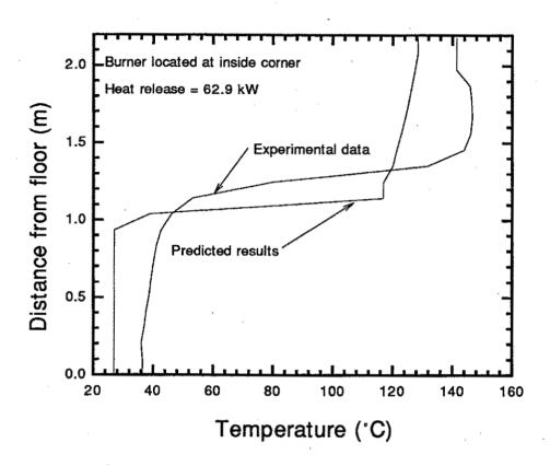
Figure 7 Comparison of predicted and experimental temperatures inside room near door.
