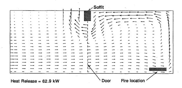
Figure 11 Velocity vectors for the door case and burner located at the inside corner.
