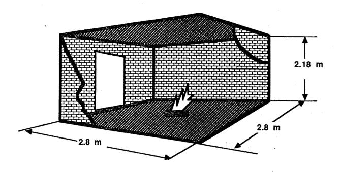
Figure 2 : Three Dimensional View of the Fire Compartment
