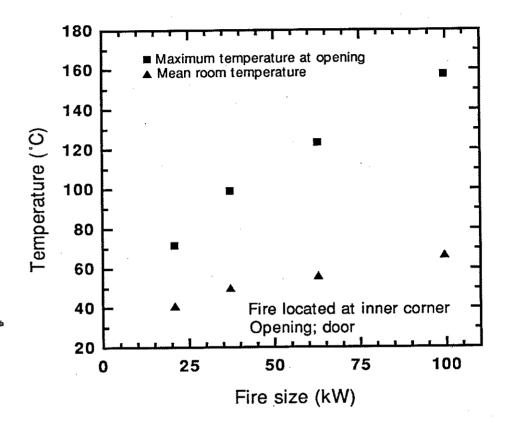
Figure 16 Predicted mean room temperature and maximum temperature at opening as a function of fire size.
