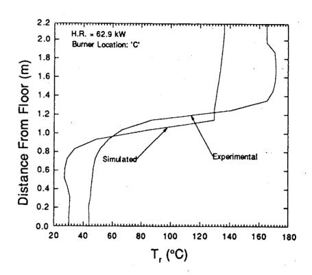
Figure 10 Comparison of predicted and experimental temperature profiles inside the room (with window opening).
