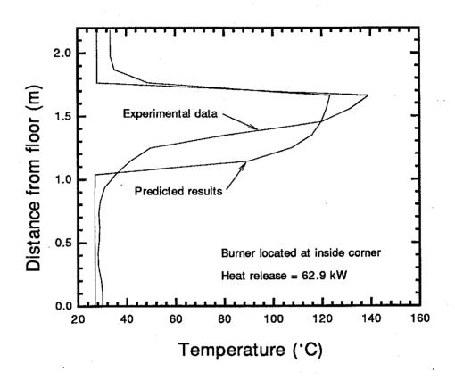
Figure 5 Comparison of predicted and experimental temperatures at the door.
