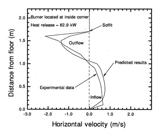
Figure 6 Comparison of predicted and experimental velocity profiles at the door.
