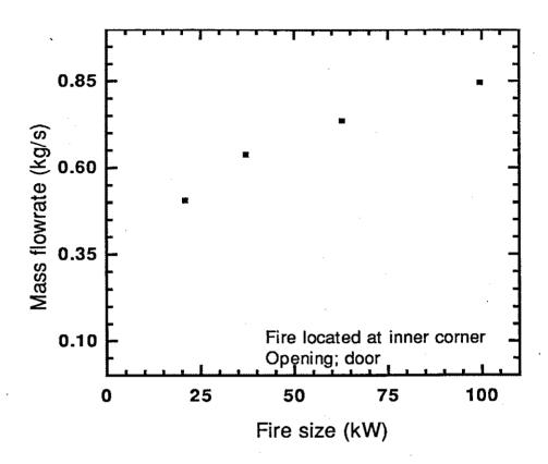
Figure 17 Predicted mass flowrate through door as a function of fire size.
