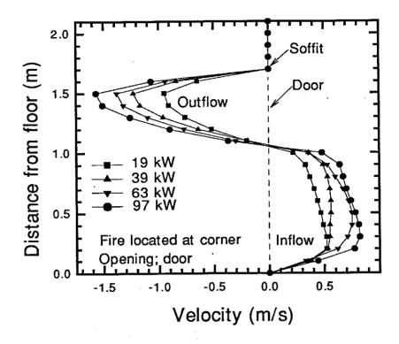
Figure 18 Predicted velocity profiles at door for various fire sizes.
