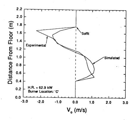
Figure 9 Comparison of predicted and experimental velocity profiles at the window.
