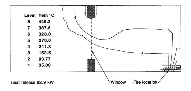
Figure 14 Temperature contours for the window case and burner located at the inside corner.
