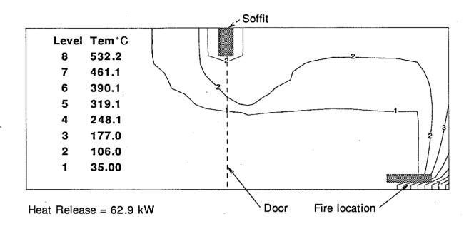
Figure 12 Temperature contours for the door case and burner located at the inside corner.
