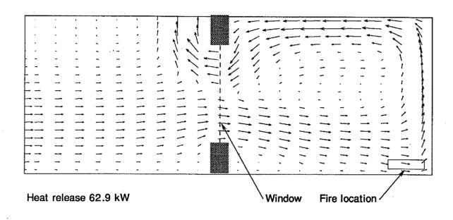
Figure 13 Velocity vectors for the window case and burner located at the inside corner.
