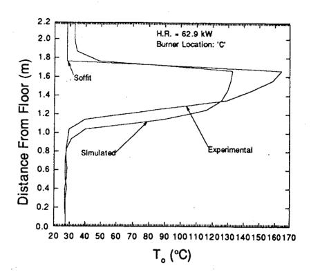
Figure 8 Comparison of predicted and experimental temperature profiles at the window.
