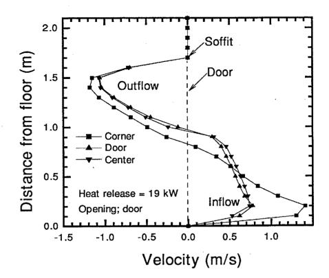
Figure 15 Predicted velocity profiles at door for various fire locations.
