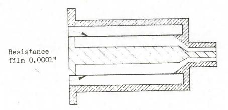
The film thickness must be less than the skin depth at frequency measured.
