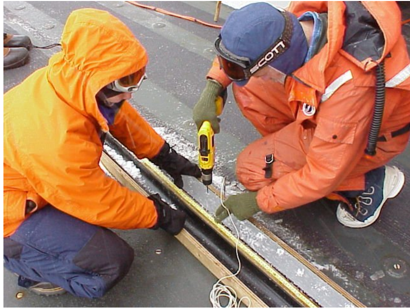
Figure 5: Photograph showing a temperature measurement on a new core
