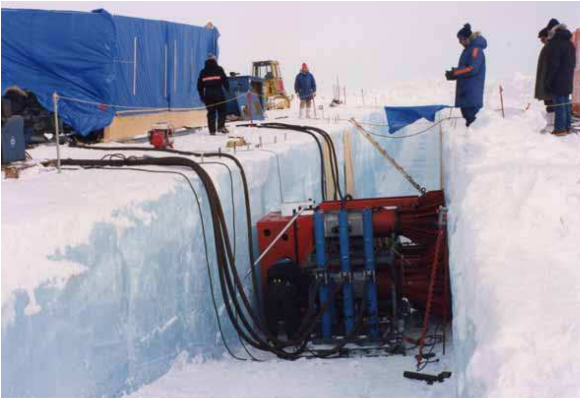
Figure 32: Ice loading apparatus in 3-m deep trench in multi-year ice.
