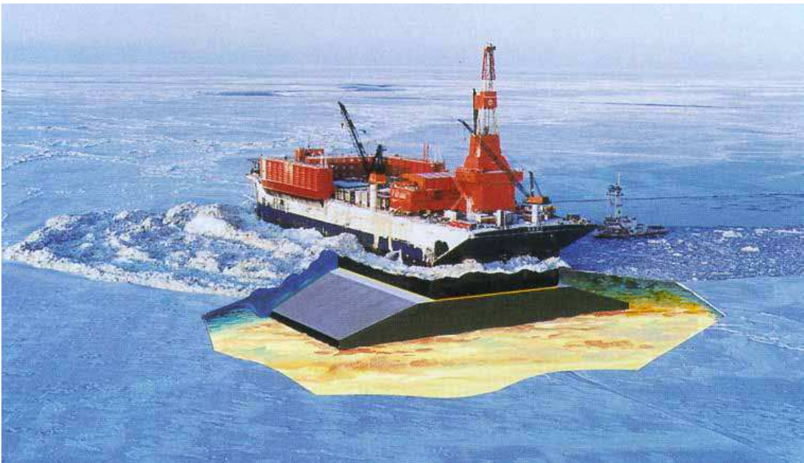
Figure 19: Cut-away view showing the SSCC and the MAT.
