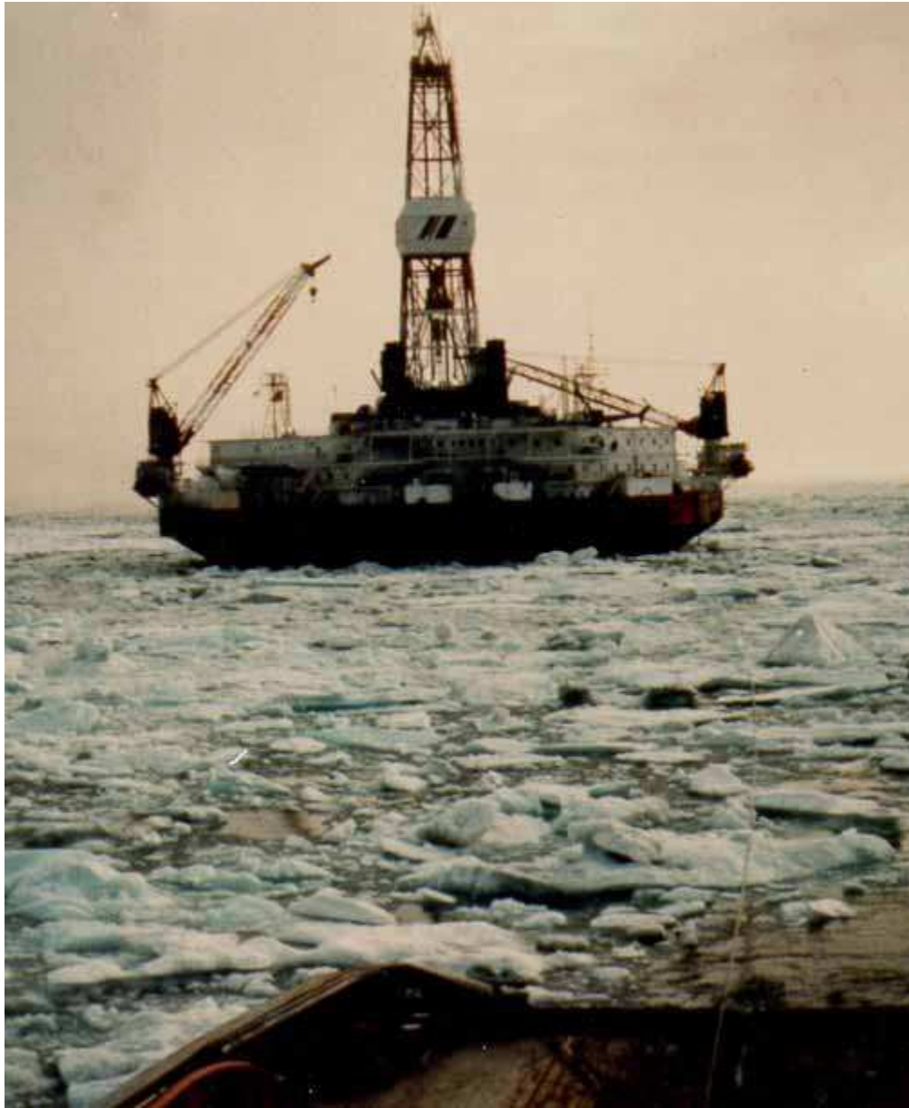
Figure 14: Kulluk in 8/10's ice under tow to a drill site.
