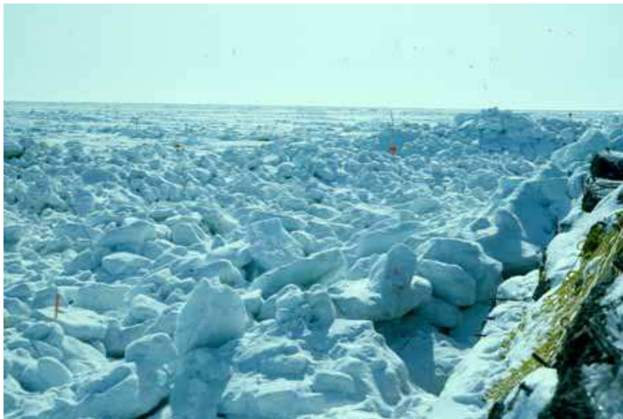
Figure 30: Photograph showing the grounded ice rubble and markers around Tarsiut where load and deformation measurements were made.
