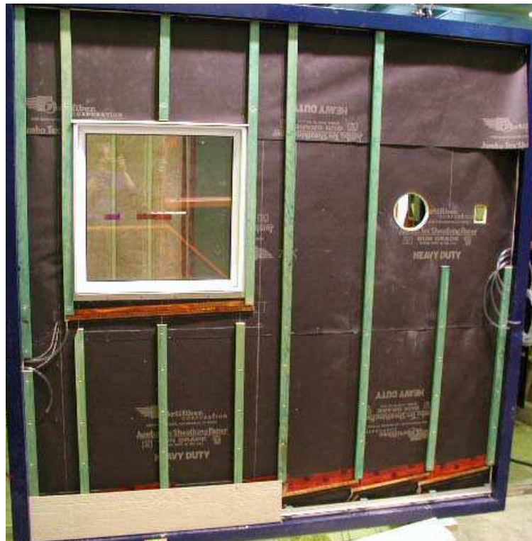
Figure A4.11 Specimen No. 16. Placement of furring strips and water collection system at the bottom of each cavity
