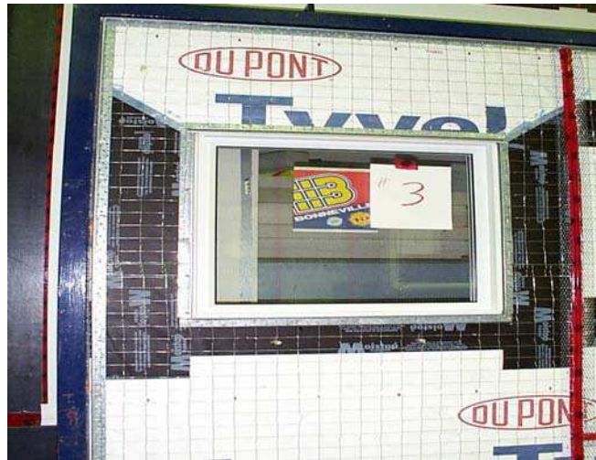
Figure 1.15. Completed window installation in specimen No. 3
