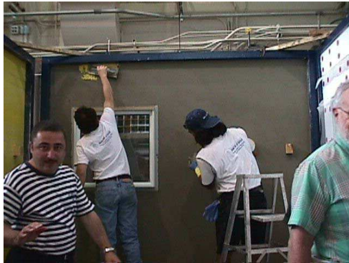
Figure 2.62. Wall No. 9. Application of WRB coating
