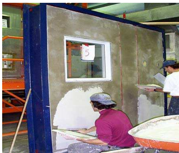
Figure 1.42. Application of the finish coat on wall No. 5.
