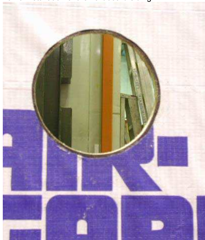
Figure A4.6 Specimen No.15. Deficiency in the installation of the WRB at the duct opening
