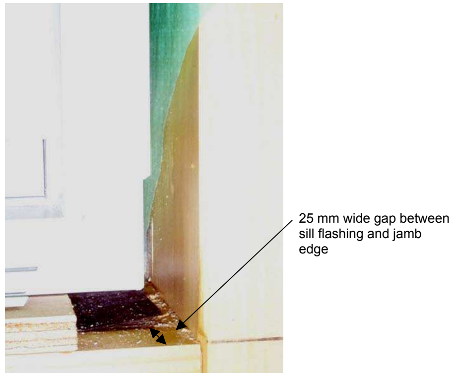
Figure 1.13. Deficiency at the sill and jamb levels for specimens No. 1 and No. 3
