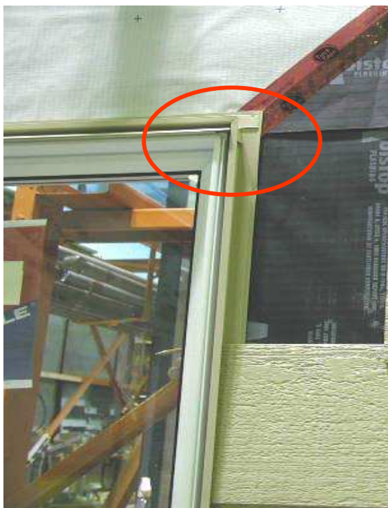
Figure A4.4. Specimen No. 15 Placement of J-trim around window
