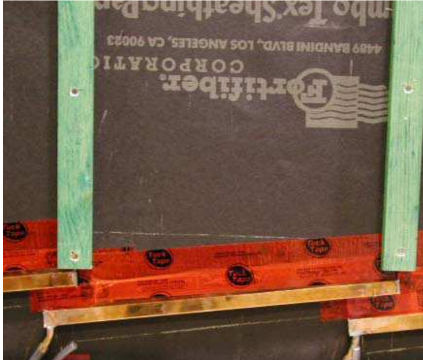
Figure A4.12 Specimen No. 16. Zoom on the water collection device at the bottom of each cavity
