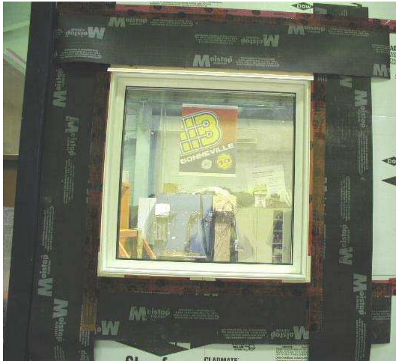
Figure A4.14 Specimen No.17. Placement of membranes around the window frame
