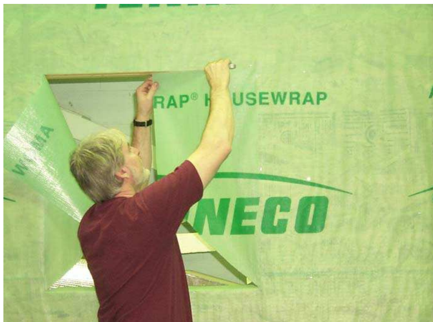
Figure 1.12. Modified I cut procedure for wall specimen No. 1
