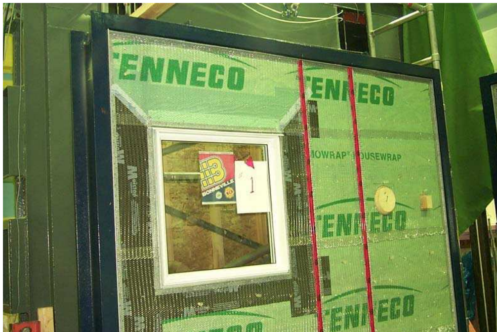
Figure 1.13. Deficiency at the sill and jamb levels for specimens No. 1 and No. 3
