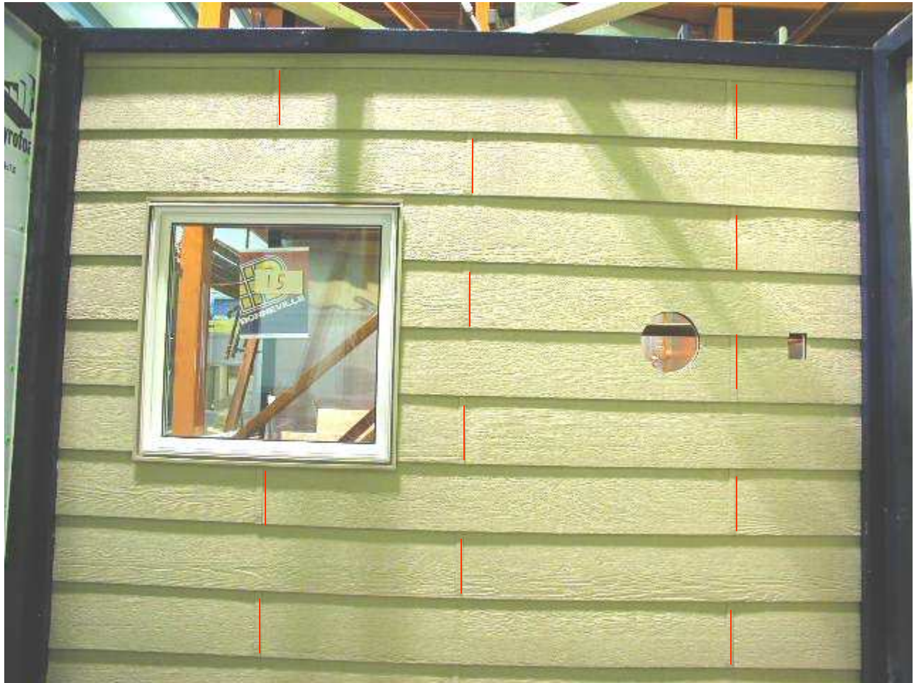
Figure A4.7 Specimen No.15. Location of the joints in the siding (same location for all 3 specimens)
