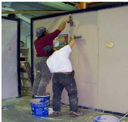
Figure 1.33. Application of the acrylic finish coat on specimen No. 4
