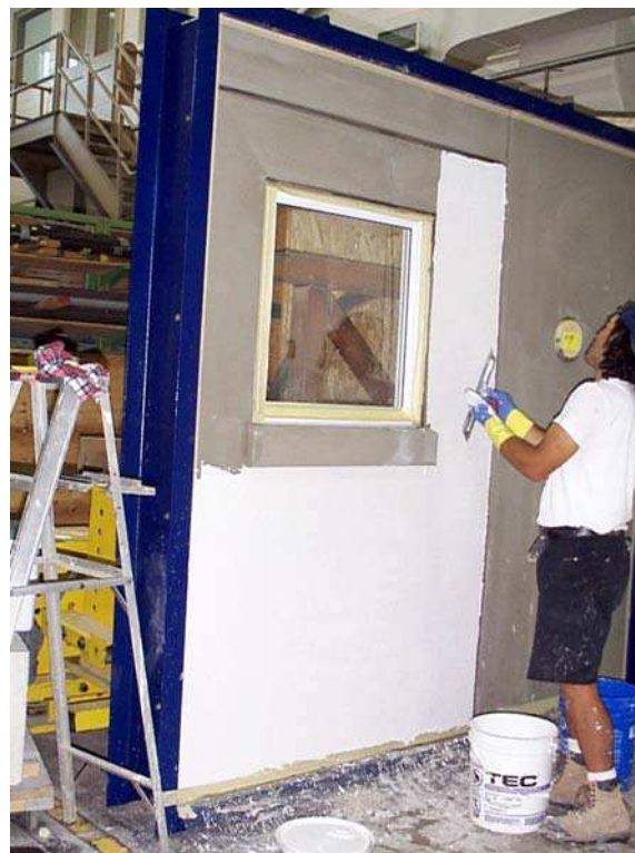
Figure 2.61. Wall No. 8. Application of finish coat
