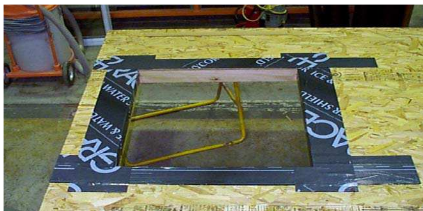
Figure 1.36. Self-adhesive flashing installed on wall specimen No. 5
