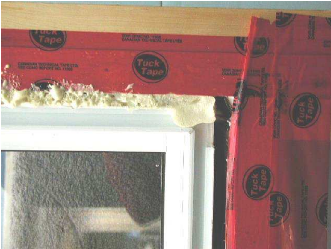
Figure A3.3 Specimen No. 11. Foaming at the window head and jambs (rough sill is left clear to place the water collection gutter)
