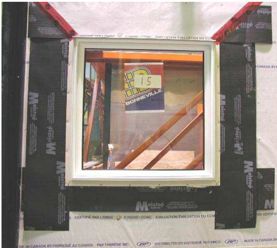
Figure A4.3 Specimen No.15. Front view of the membranes installed around the window (left) according to Dupont procedure (right)
