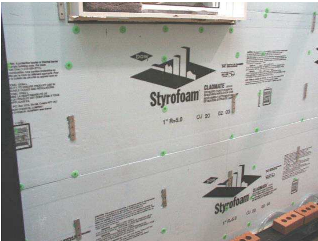
Figure A3.1 Installation of the foam sheathing on specimen No. 11
