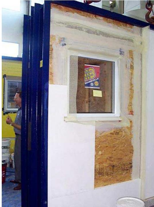
Figure 2.48. Wall No. 6. Installation of EPS insulation
