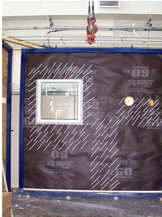
Figure 2.52. Wall No. 7. WRB membrane with water sensitive paper strips
