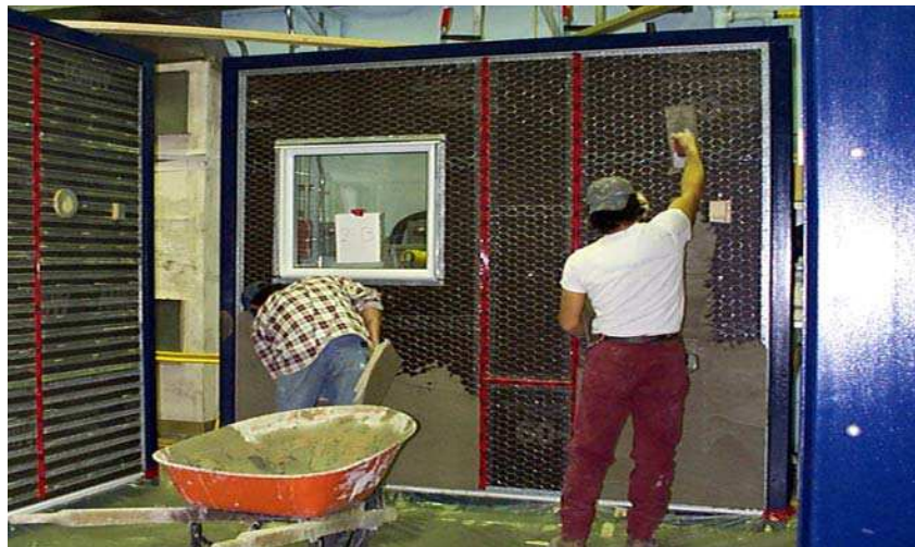
Figure 1.29 Application of the scratch coat on specimen No. 2b
