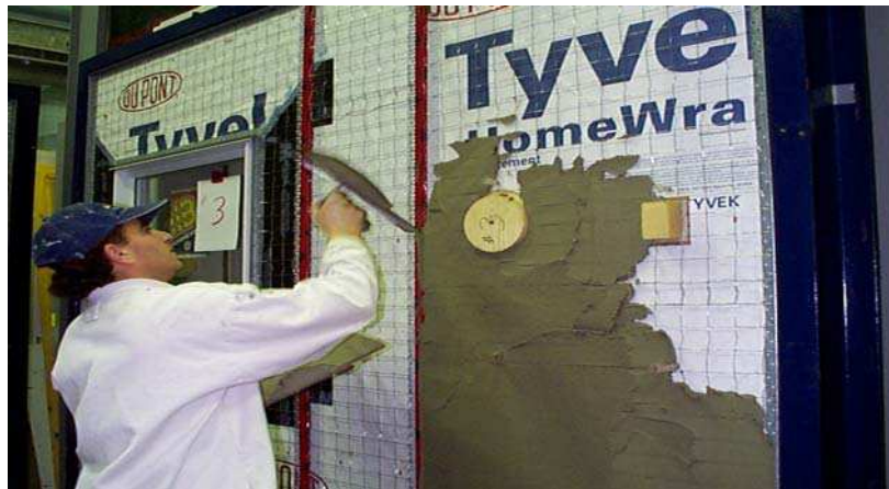
Figure 1.28. Application of the scratch coat on specimen No. 3
