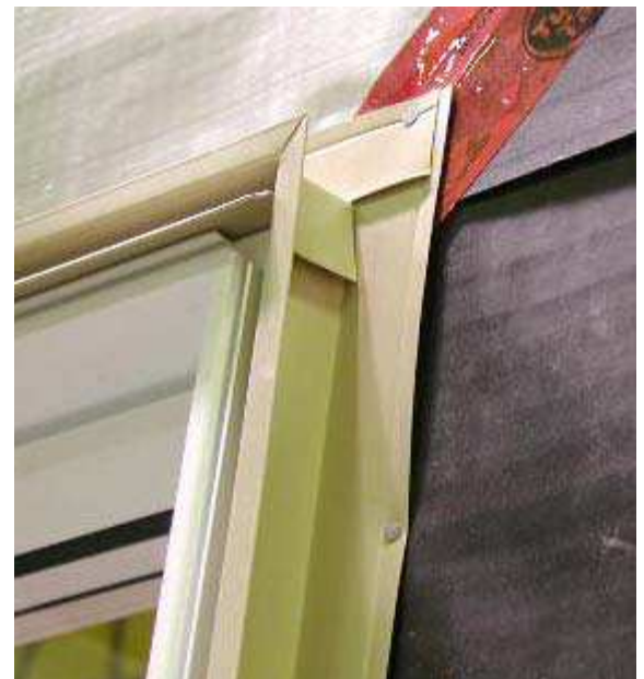
Figure A4.3 Specimen No.15. Front view of the membranes installed around the window (left) according to Dupont procedure (right)
