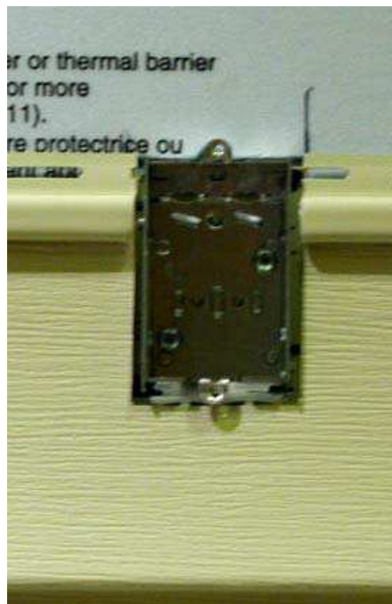
Figure A4.17 Specimen No 17. Installation of the electrical outlet
