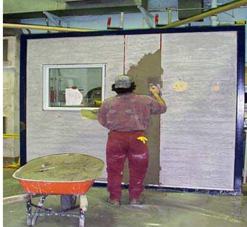
Figure 1.31. Application of the brown coat on wall specimen No. 2b
