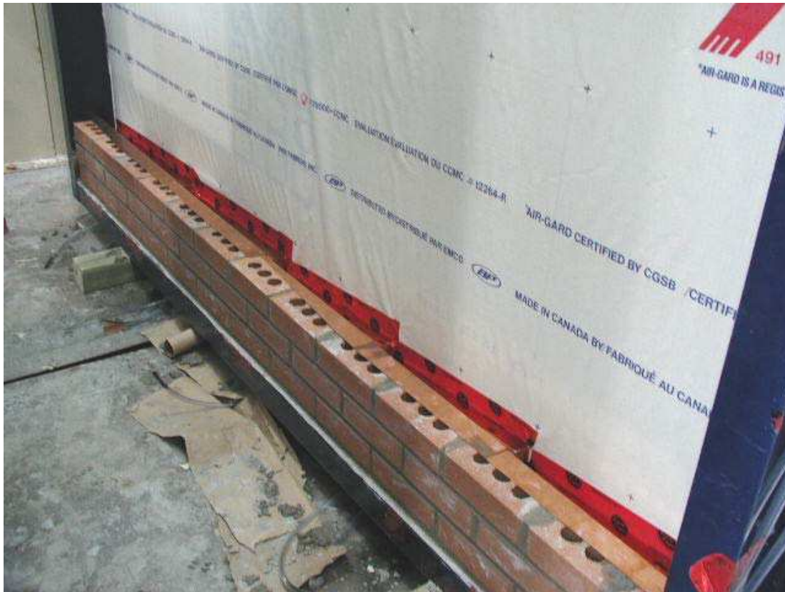
Figure A3.20 Installation of the water collection roughs at the bottom of the specimen No. 14
