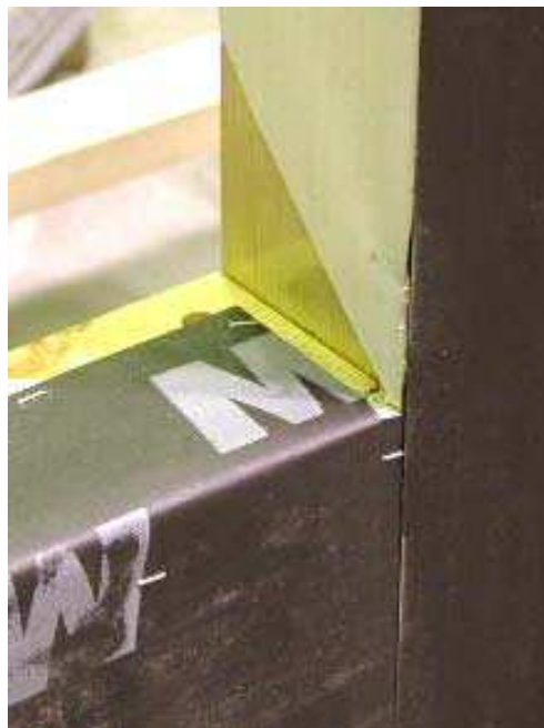
Figure A4.2 Specimen No.15. Close-up on the deficiencies at the rough sill
