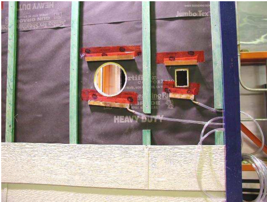
Figure A4.10 Specimen No.16. Detailing at the ventilation duct and outlet, showing the gutter system placed for water collection
