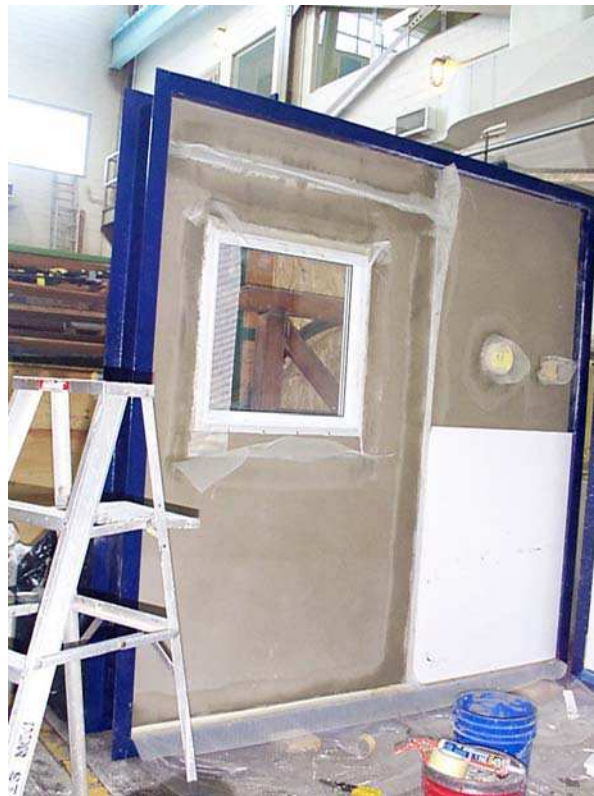
Figure 2.59. Wall No. 8. Backwrapping and installation of adhered EPS insulation
