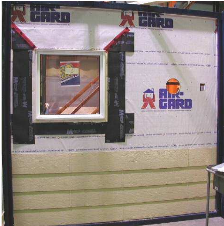
Figure A4.5 specimen No.15 Installation of the hardboard siding
