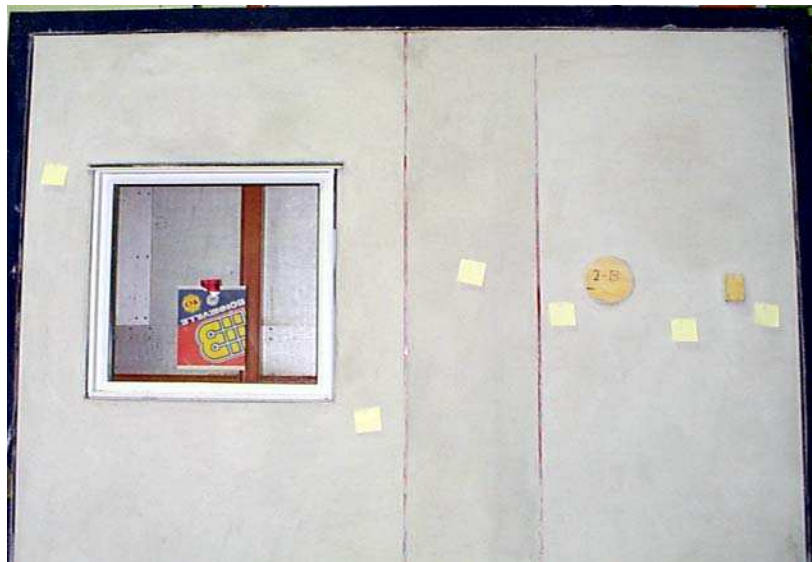
Figure 1.46. Cracks in specimen No. 2b covered for 15 days
