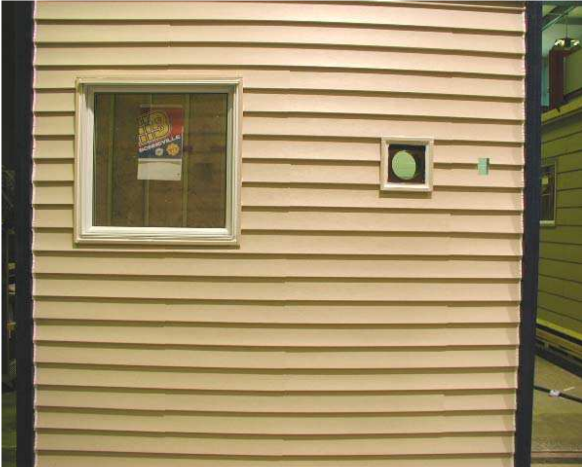
Figure A4.18 Specimen no 17. Installation of vinyl siding completed
