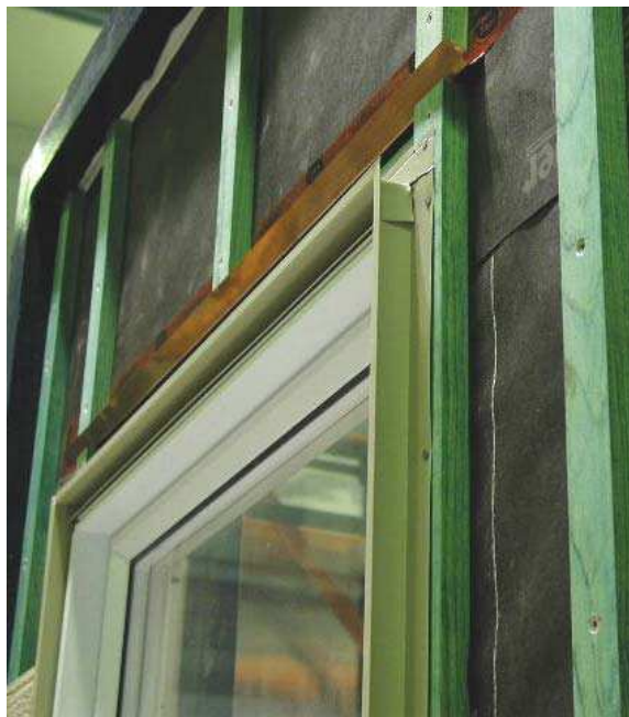
Figure A4.9 Specimen No.16. Zoom on the detailing at the window head
