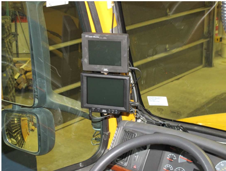
Figure 19: Monitors mounted in subject vehicle on left A-pillar
