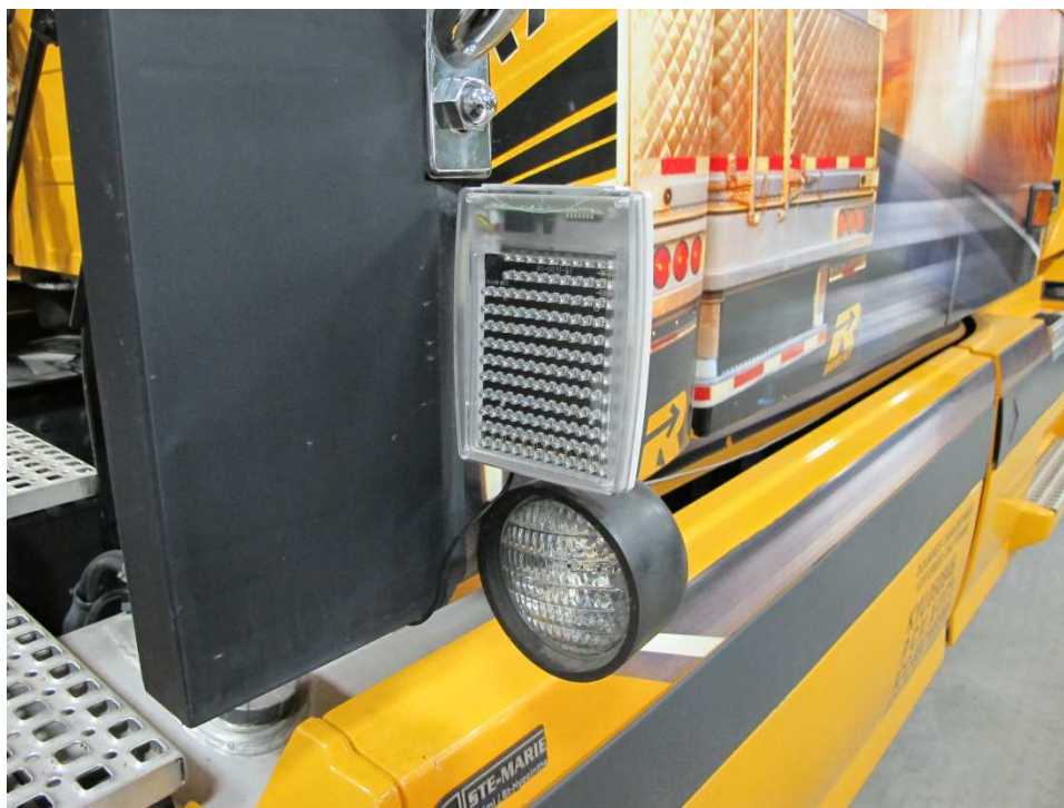
Figure 22: IR illuminator mounted on the side of the subject vehicle
