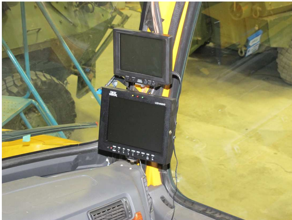
Figure 20: Monitors mounted in subject vehicle on right A-pillar
