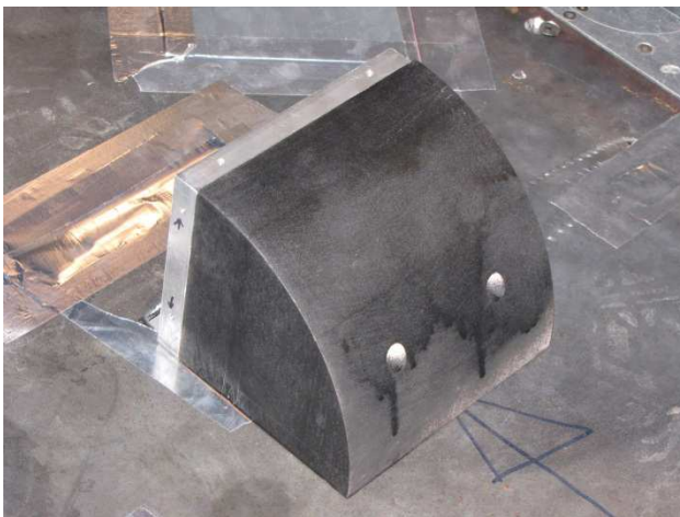
Figure 30: IR illuminator prototype fairings in the wind tunnel
