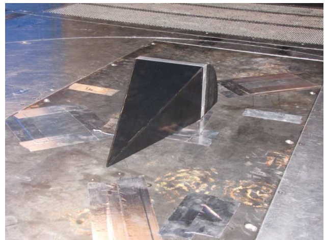
Figure 30: IR illuminator prototype fairings in the wind tunnel
