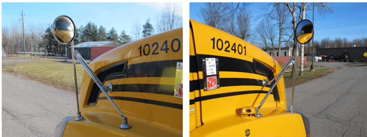
Figure 12: Fender-mounted convex mirrors on subject vehicle
