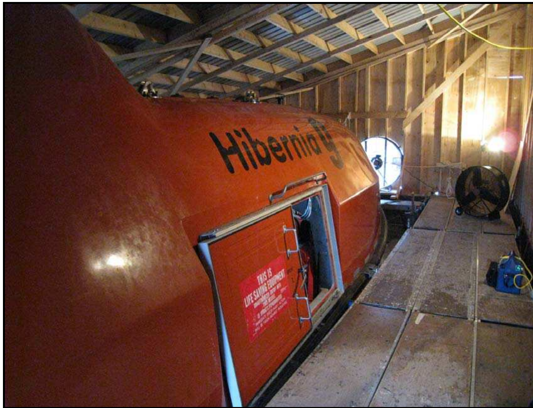
Figure 3. Experimental setup of a 72-person SOLAS lifeboat
