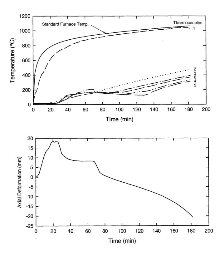
Figure A5. Temperatures and axial deformation of Column No. C-66
