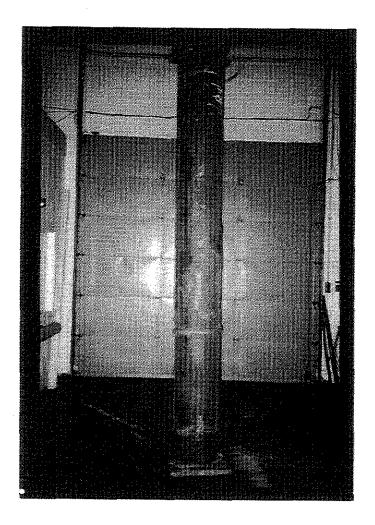
Figure B.3. Column No. C-58 after fire test
