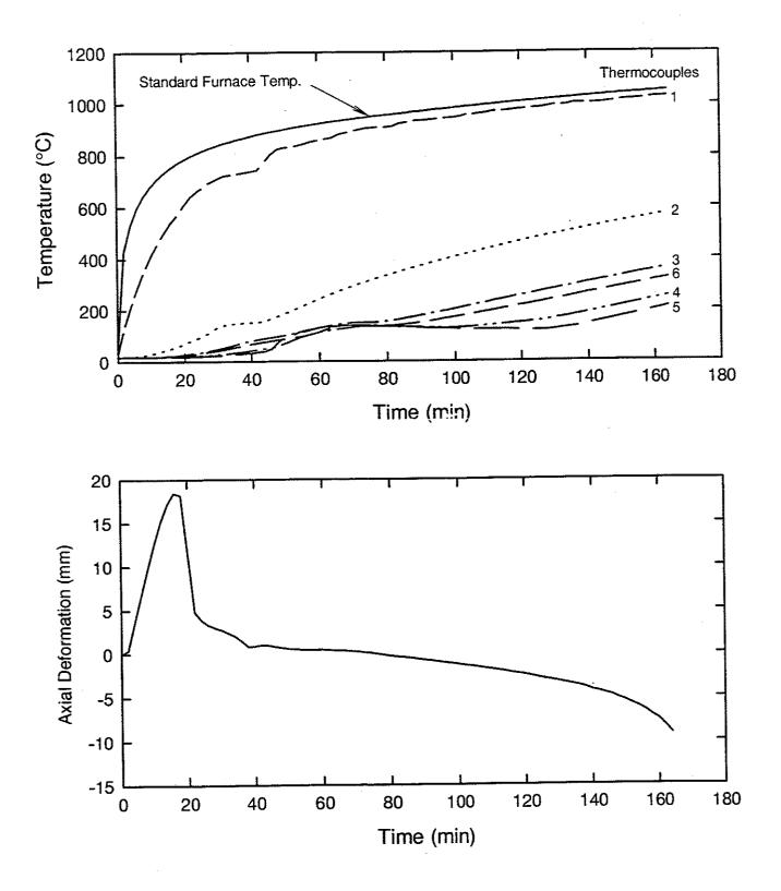
Figure A1. Temperatures and axial deformation of Column No. C-52
