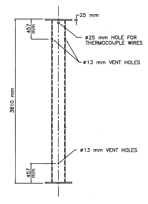
Figure 1. Elevation and cross-sectional details of a typical column
