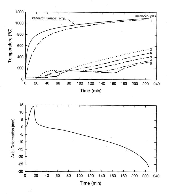
Figure A6. Temperatures and axial deformation of Column No. C-67
