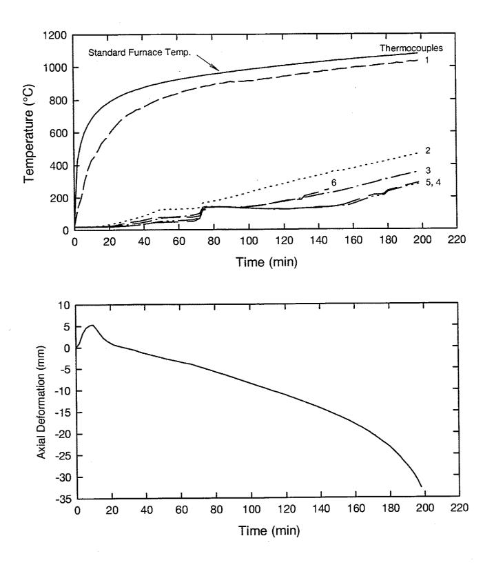
Figure A4. Temperatures and axial deformation of Column No. C-65
