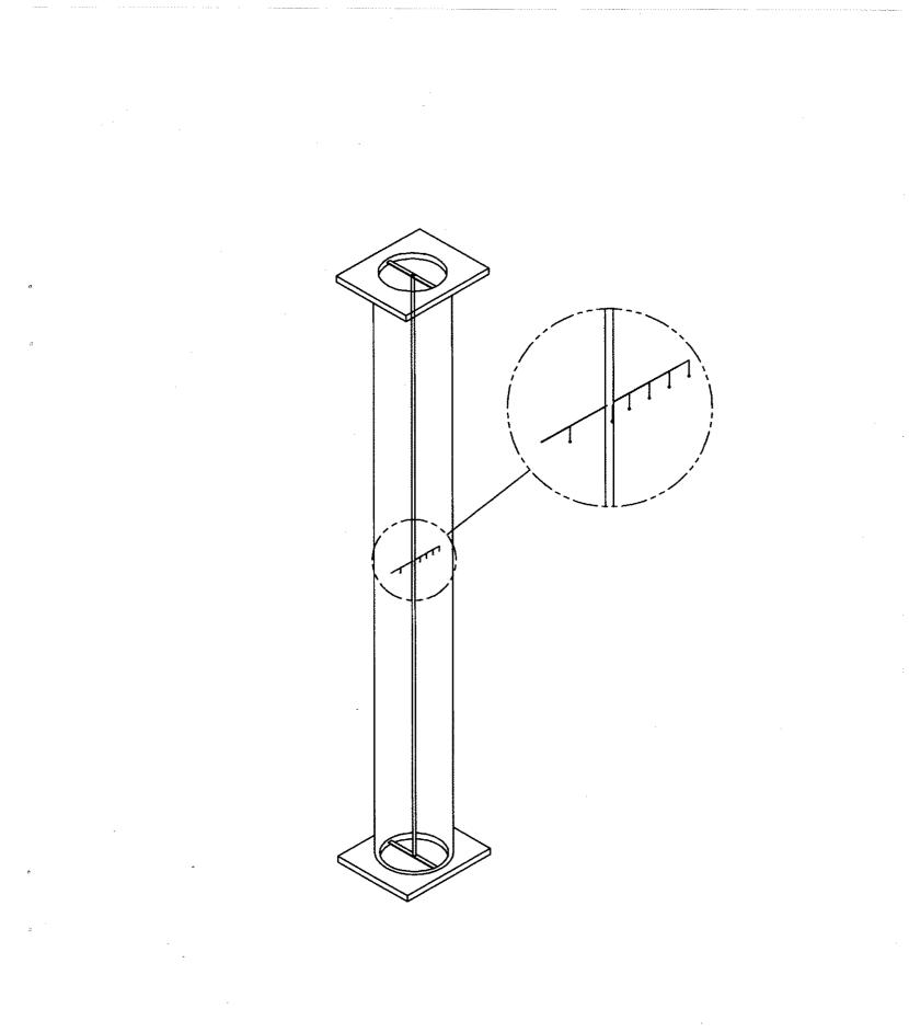
Figure 3. Layout of thermocouple frame in a column
