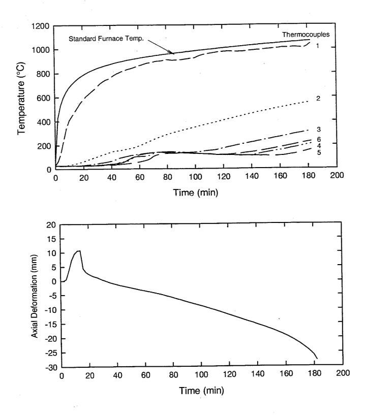
Figure A2. Temperatures and axial deformation of Column No. C-54
