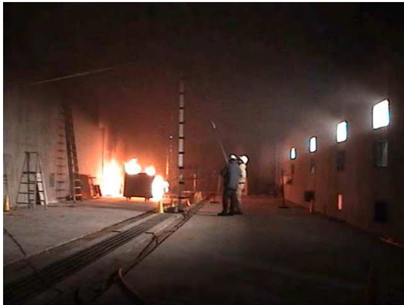
Figure 6.4. Tunnel conditions with a gasoline pool fire (1.0 m x 1.0 m) underneath the vehicle in test T-7
