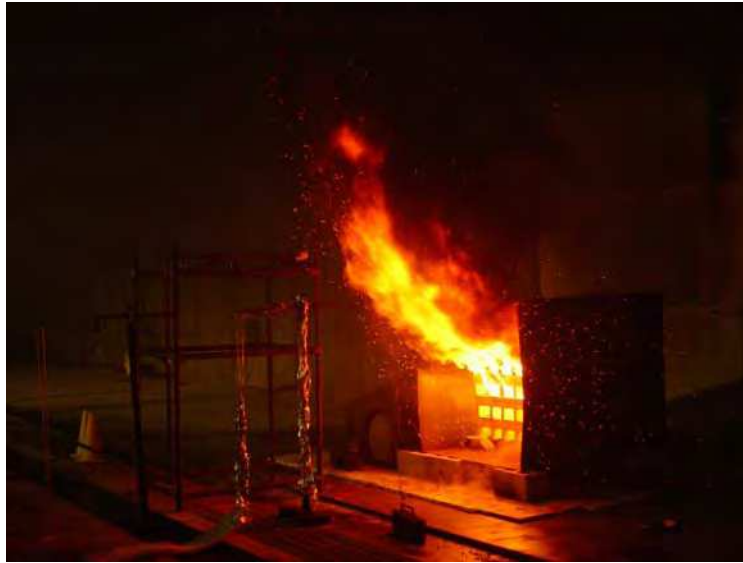
Figure 6.38. Passenger compartment fire with wood cribs in test T-14
