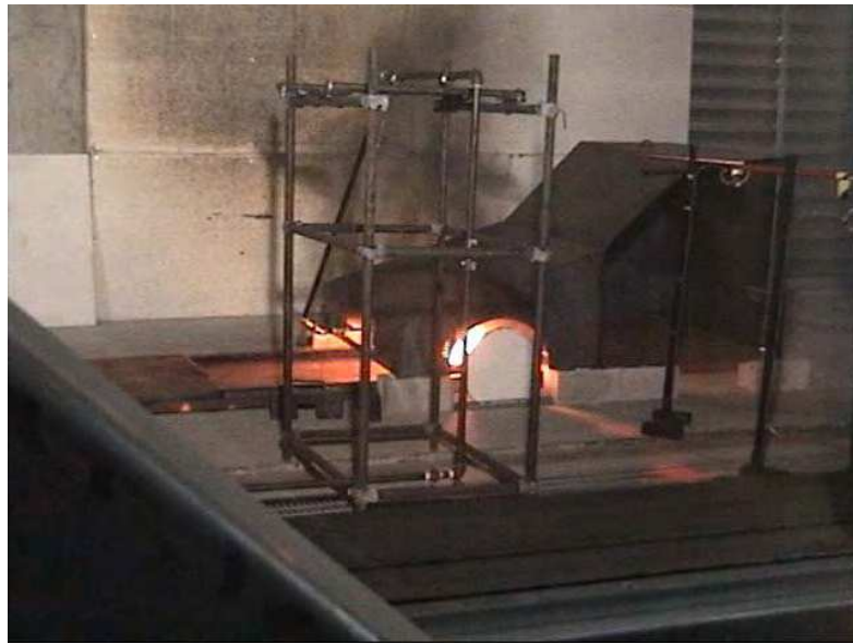
Figure 6.3. A 0.3 m x 0.3 m gasoline pool fire underneath the vehicle in test T-2
