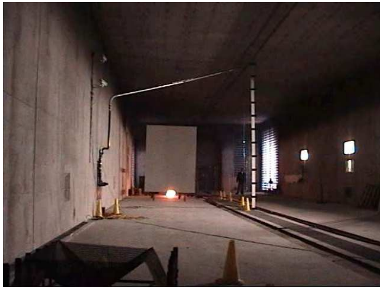
Figure 6.22. Front view of a 0.09 m 2 gasoline pool fire behind a large vehicle (T-8)
