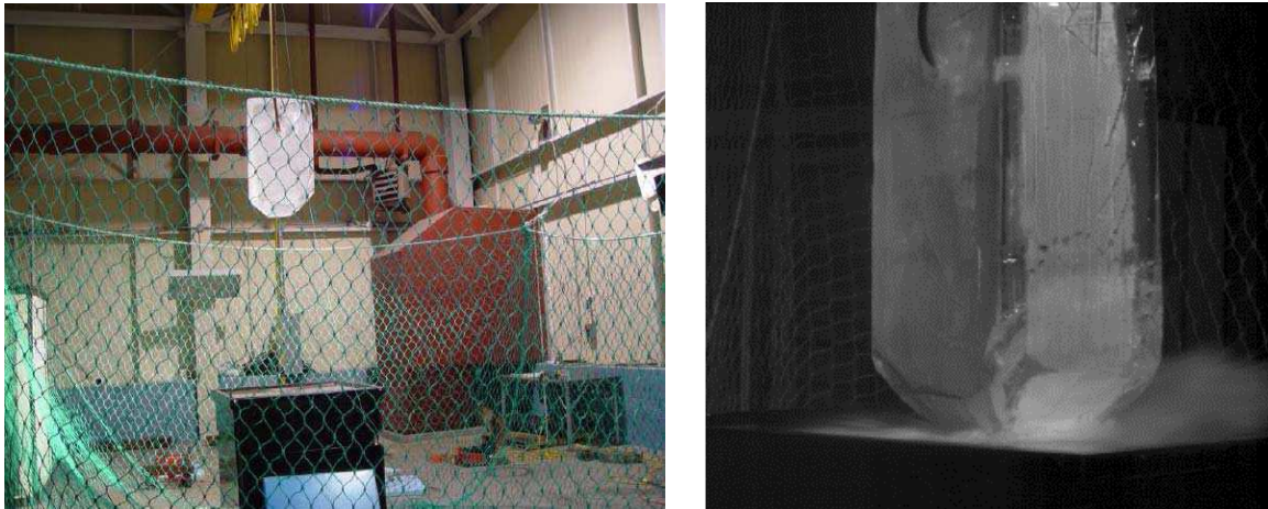
Figure 1: Ice drop testing with large-scale impact module (Gagnon, et al. 2009)
