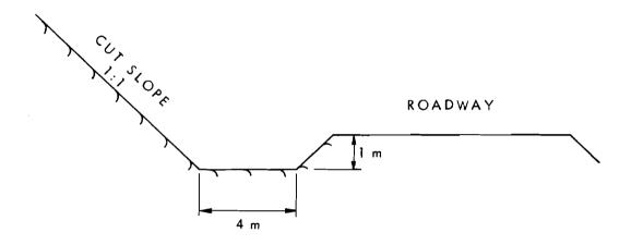
The method could be applied at slopes not higher than 15 m and at locations where it would be easy to obtain the additional width of cross section.
