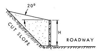
The space behind the barrier, height H, must be sufficient to store the expected volume of avalanche snow and snow deposited by snow blowers. The volume of avalanche snow A is:
