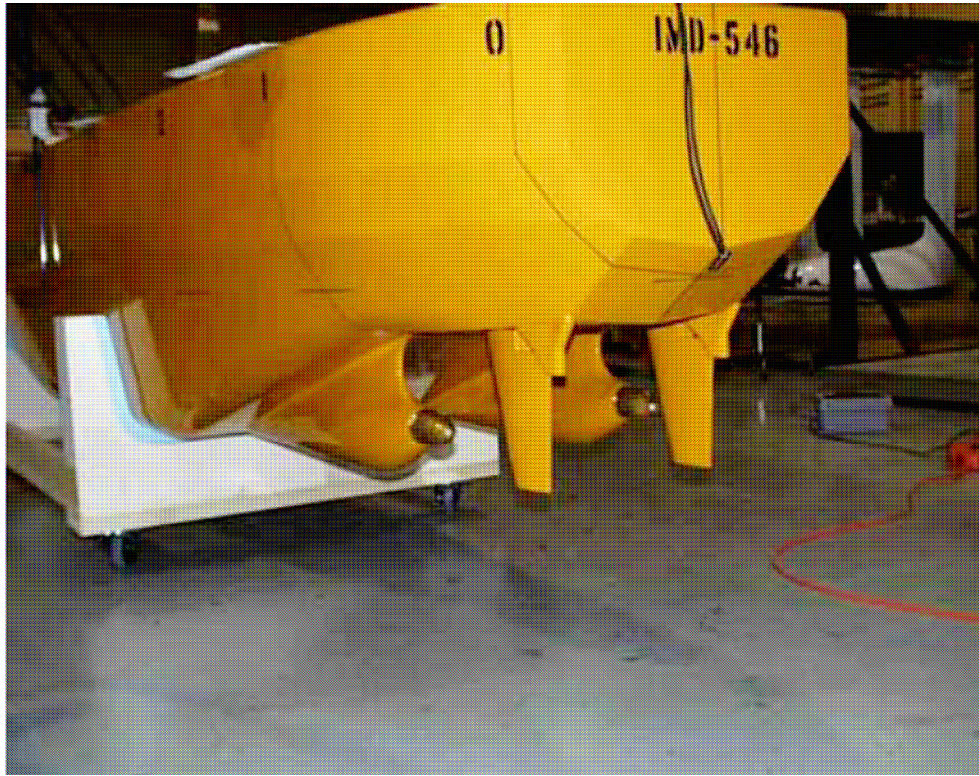
Figure 3. The stern arrangement of the Healy Model 546
