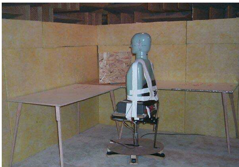
Figure 3: The B&K Head and Torso simulator (HTS) sound source in position for measurements.
