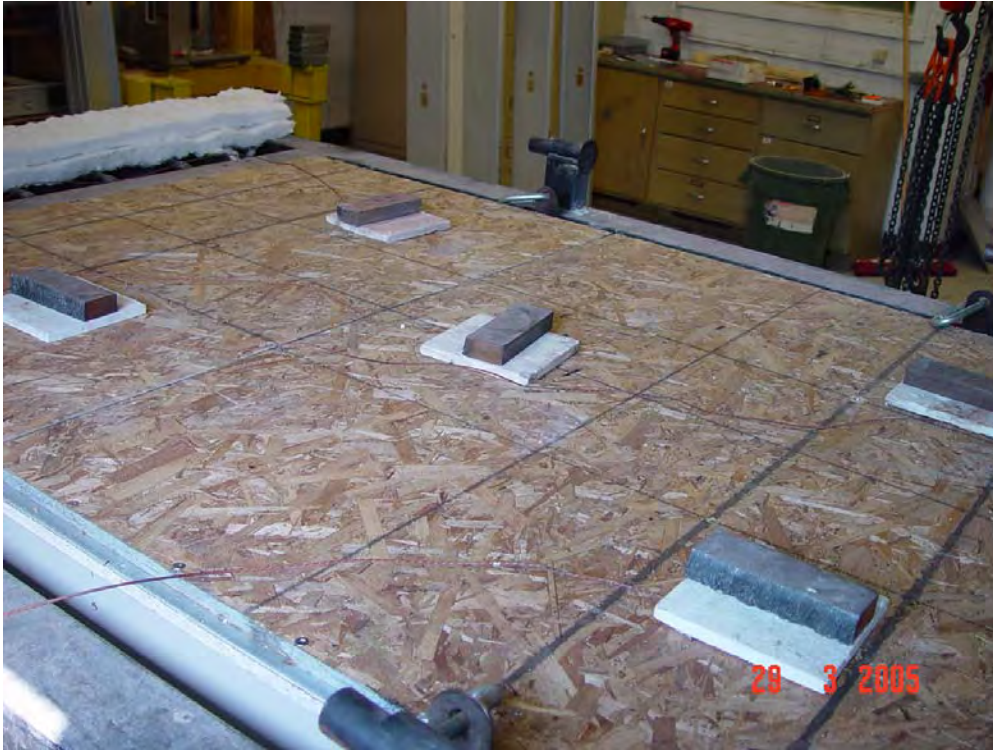
Figure C12. Typical floor assembly with tongue and groove joint (Test OSB-01A).
