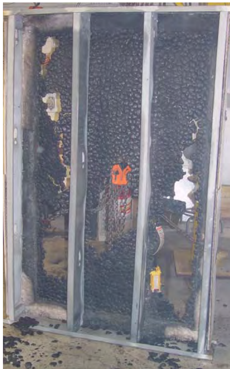
Figure C19. Damage to exposed side of test assembly (Test OSB-02B).
