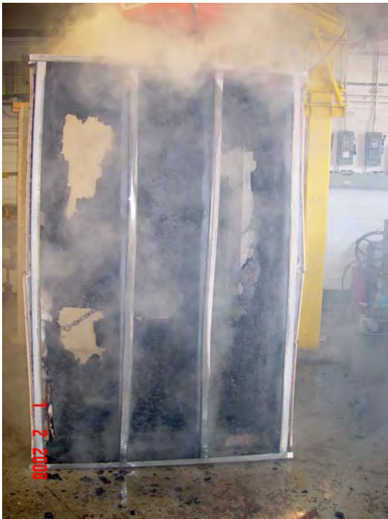
Figure D5. Flame damage Test OSB-03G.
