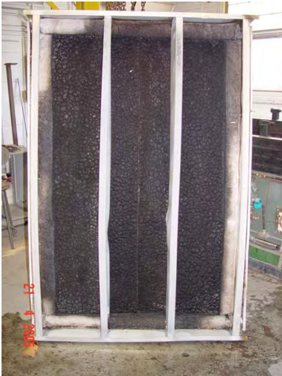
Figure D9. Flame damage Test OSB-03C.
