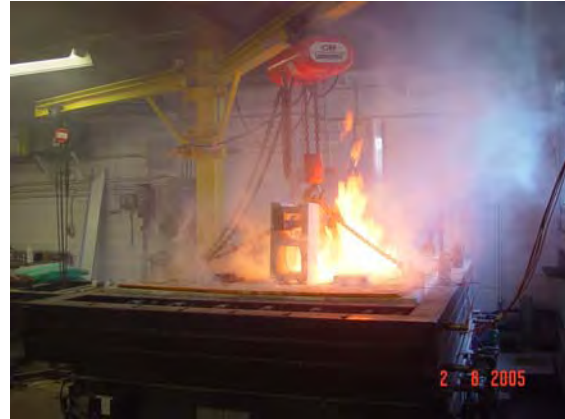
Figure D12. Flame penetration Test OSB-03D.
