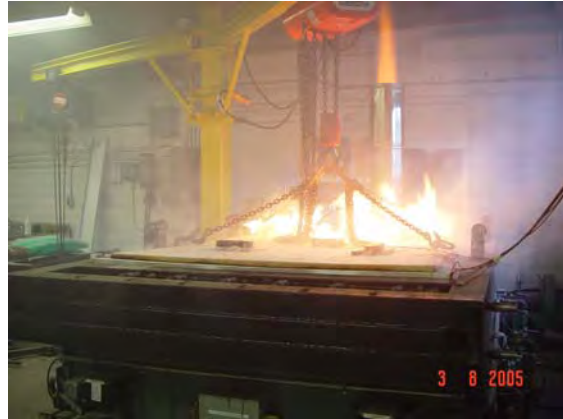
Figure D16. Flame penetration Test OSB-03E.
