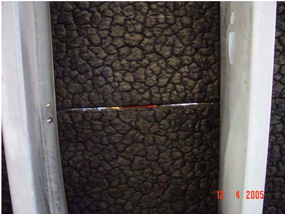
Figure C15. Damage to exposed side of floor assembly (Test OSB-03A).
