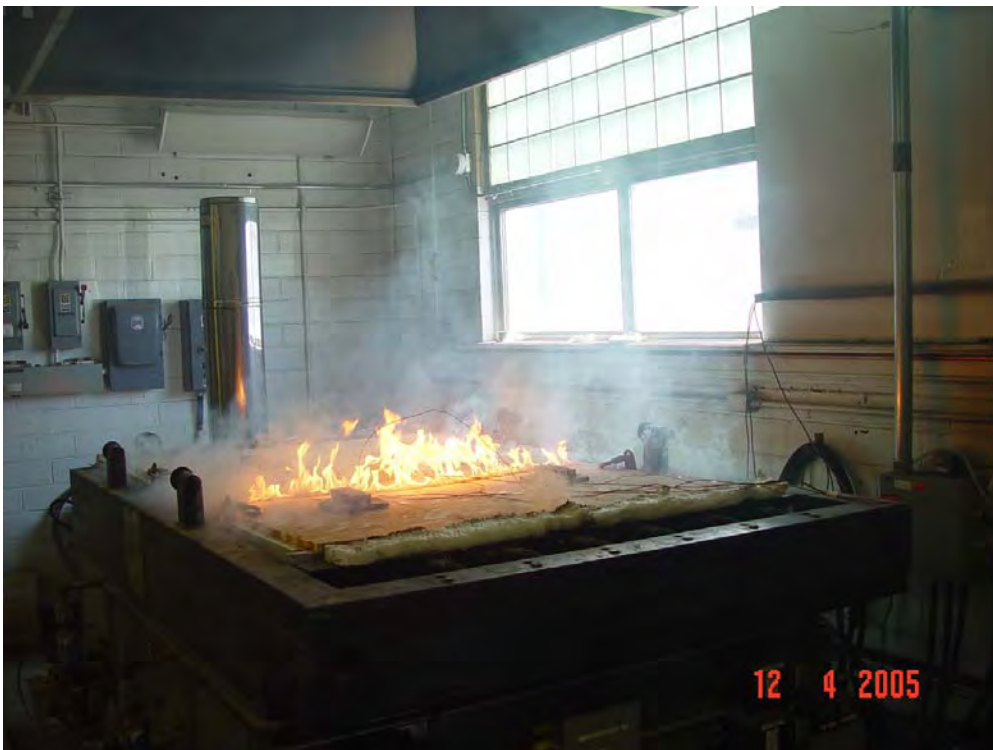
Figure C13. Flame penetration through tongue and groove joint (Test OSB-03A).
