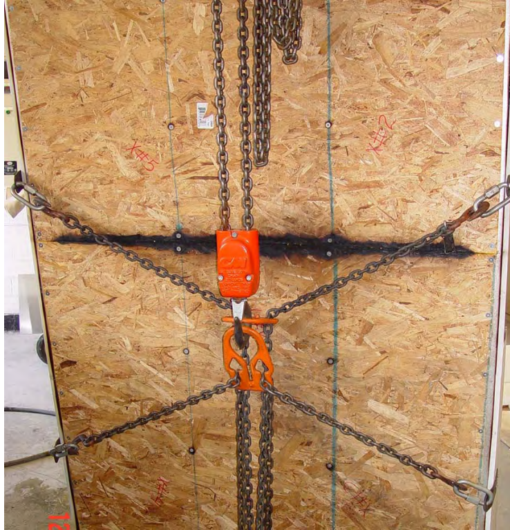
Figure C14. Damage to unexposed side of floor assembly (Test OSB-03A).
