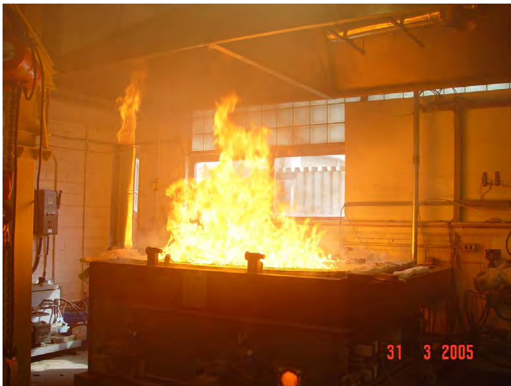
Figure C17. Flame penetration through test assembly (Test OSB-02B).
