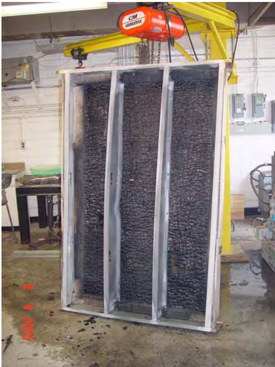
Figure E9. Flame damage Test PLY-01B.
