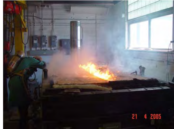
Figure D8. Flame penetration Test OSB-03C.
