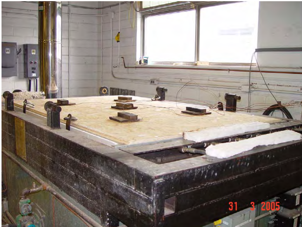
Figure C16. Typical floor assembly with full OSB panel (Test (OSB-02B)).
