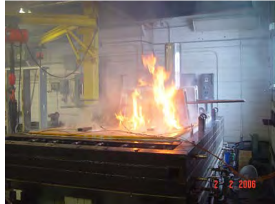
Figure D28. Flame penetration Test OSB-03H.
