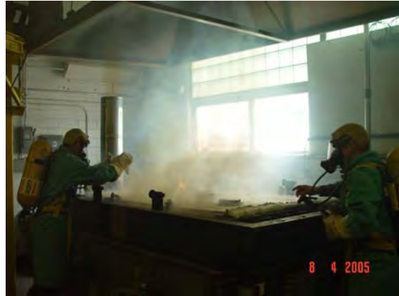
Figure E8. Flame penetration Test PLY-01B.
