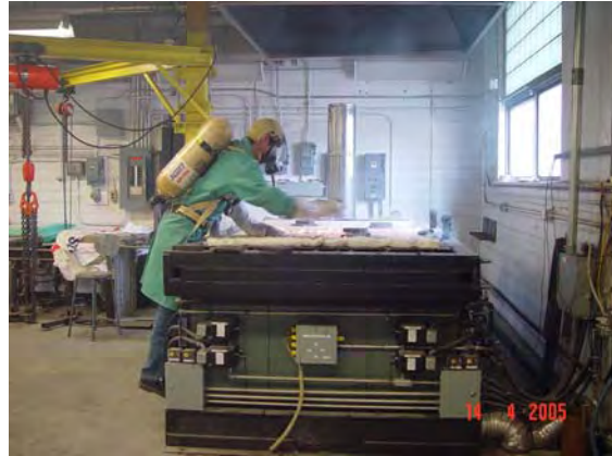
Figure E4. Flame penetration Test PLY-01A.
