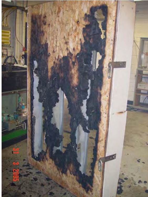
Figure C18. Damage to unexposed side of test assembly (Test OSB-02B).
