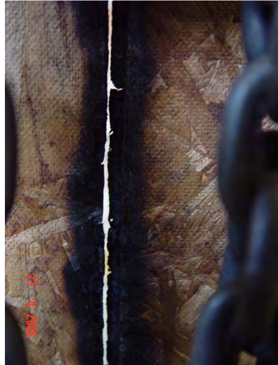
Figure D10. Damage joint Test OSB-03C.
