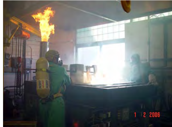
Figure D24. Flame penetration Test OSB-03G.
