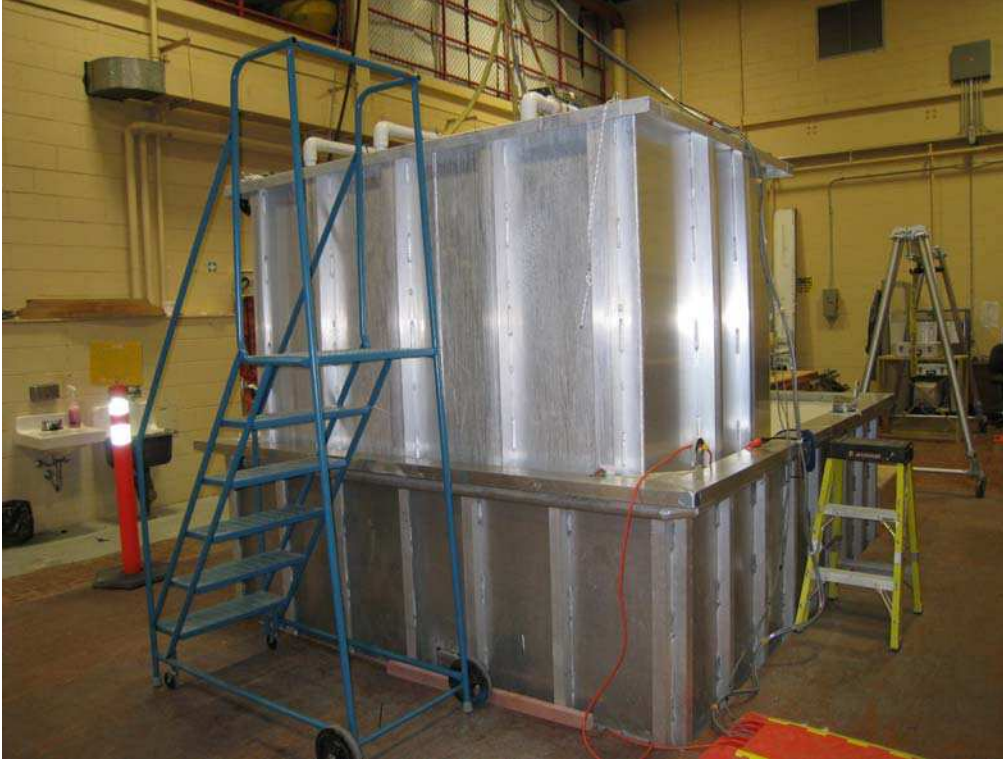
Figure 4. Aluminum tank for thermal manikin tests
