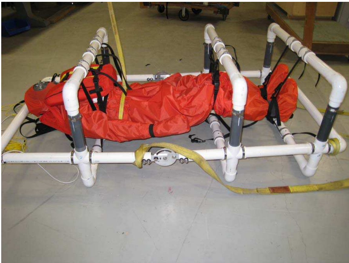
Figure 7. Manikin flotation position matched in a frame on land
