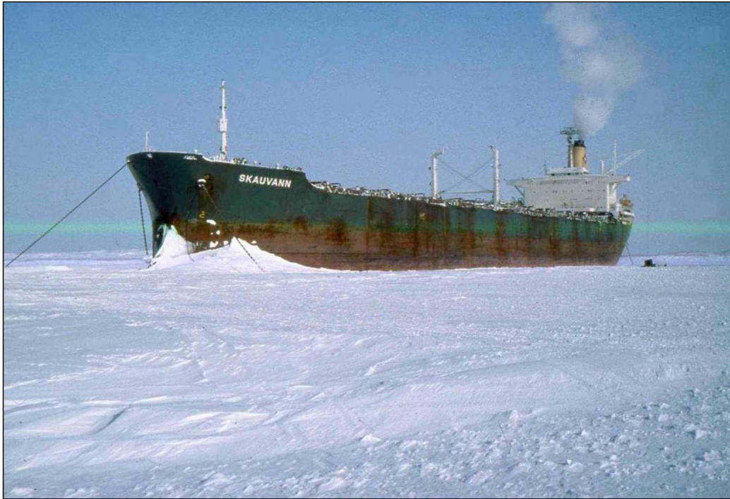
Figure 6: Tanker “Skauvann” overwintering fuel storage in Wise Bay in the 1980’s (from Connelly, 2012). The tanker maintained a crew onboard year-round.
