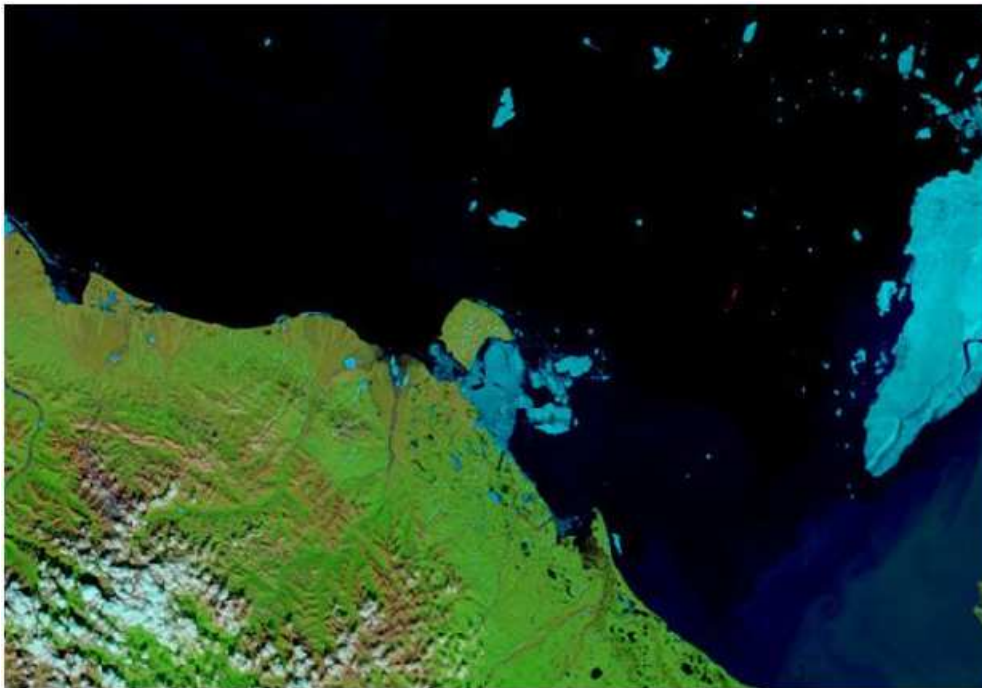
Figure 14: MODIS satellite image showing the break-up of ice in the bay around Herschel Island. This break-out of ice presents a moving ice situation which will exert ice loads on a moored vessel. Image from June 29, 2009, Terra satellite, Bands 7-2-1 colouring.
