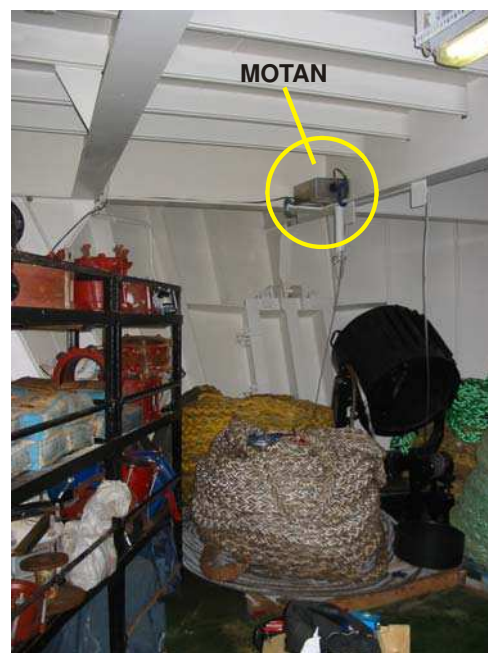
Figure 11 AutoMOTAN on the M/T Véga Desgagnés , in an area of the bow not designated as intrinsically safe
