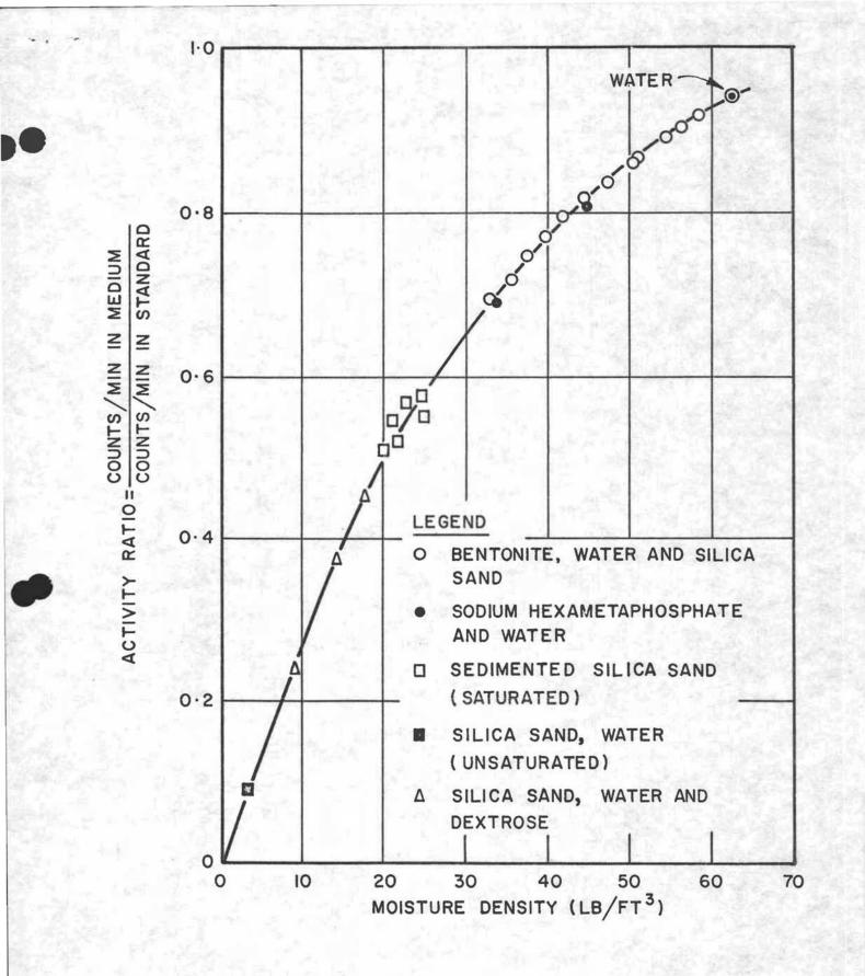
FIGURE I CALIBRATION CURVE OF NEUTRON MOISTURE METER
