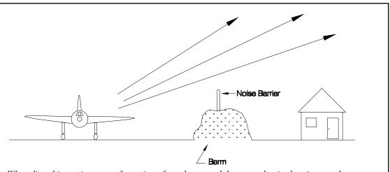
When disturbing noise comes from aircraft on the ground, berms and noise barriers can be constructed to block the direct path of the sound. They are most effective if they are located either close to the noise source or close to the home.
