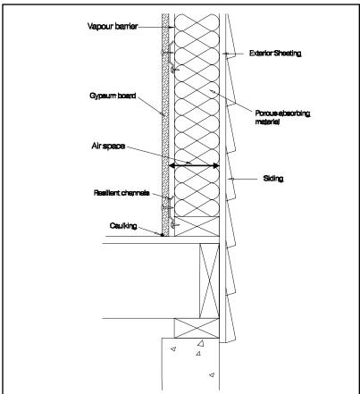
There are 5 key factors to creating a construction that is an effective barrier to sound. (1) the outer layers must be heavy, (2) there should be a vibration break between the two external surfaces, (3) porous absorbing material is needed in the cavity, (4) all cracks and holes must be sealed, and (5) there should be a large air space between the interior and exterior layers.
