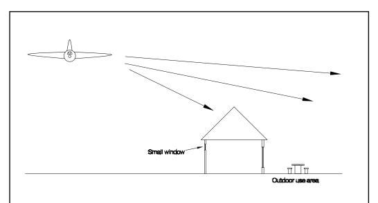
When the main aircraft flight track is on one side of the home, the building layout should be optimised to minimize noise disturbance. On the noisy side windows should be smaller. Noise sensitive rooms such as bedrooms and outdoor use areas should be located on the quiet side.
