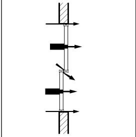
Typical vertical sliding window with double thermal glazing. Aircraft noise enters via various air leaks and the closely spaced thermal glazing is a poor barrier to low frequency helicopter and aircraft noise.
