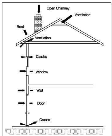
Aircraft noise can enter a building by both airborne and structure borne paths. Some airborne paths can be blocked or sealed. Ventilation openings can be treated. Structure borne paths, such as walls, windows, doors and roofs can be improved by making the construction a better barrier to sound.
