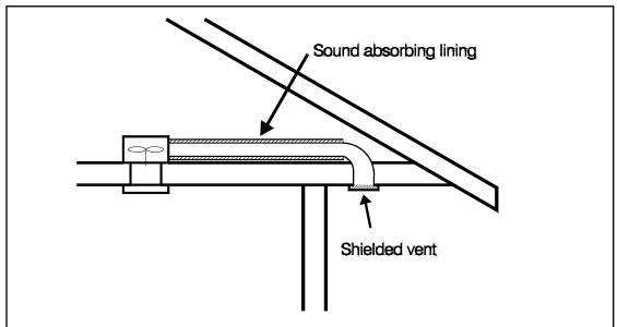
Improving the sound insulation associated with a bathroom exhaust fan by locating the vent under the eaves where it is shielded from aircraft noise and by using ducts that are lined with sound absorbing material to reduce noise transmission.
