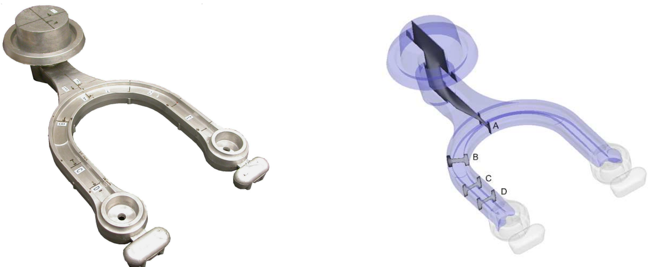
Figure 1: Typical suspension part and sampling sections
