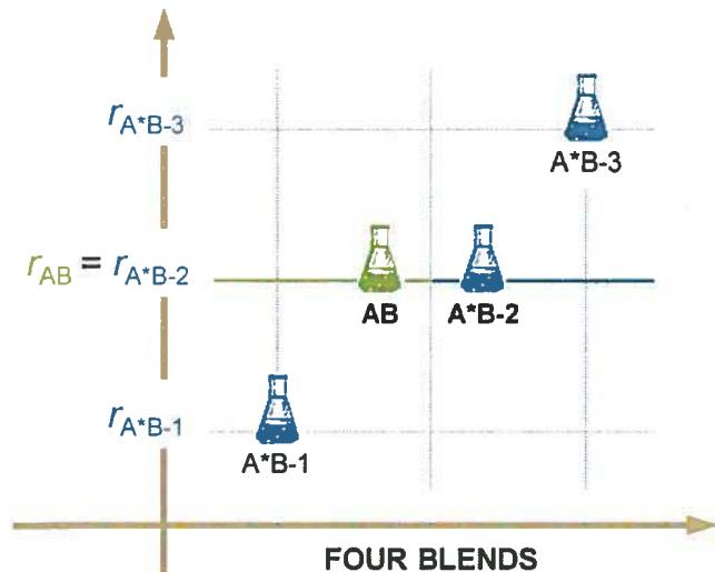
**Fig. 1.** Exact-matching quadruple isotope dilution. The isotopic ratio of the sample blend (AB) is matched to one of the standard blends ( $A^*B-2$ ), while the remaining two standard blends ( $A^*B-1$  and  $A^*B-3$ ) are chosen to bracket this isotope ratio.
