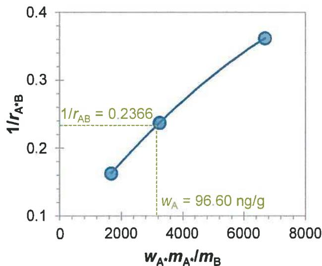
**Fig. 2.** Graphical solution of the isotope dilution challenge based on a nonlinear least square fit.
