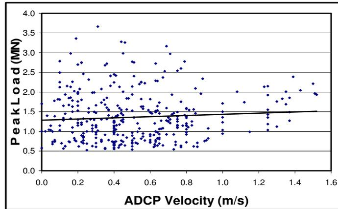
Figure 1b. ADCP Velocity Vs Peak Load for Keel Depth Range of  $H_k < 10$
