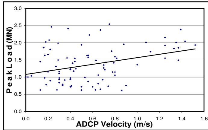
Figure 1a. ADCP Velocity Vs Peak Load for Keel Depth Range of  $H_k < 4m$
