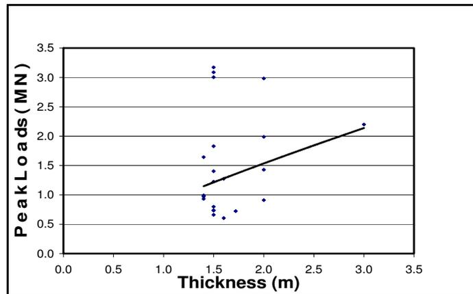
Figure 4b. Consolidated Layer Thickness Vs Load for a Range of  $H_c > 1.4m$
