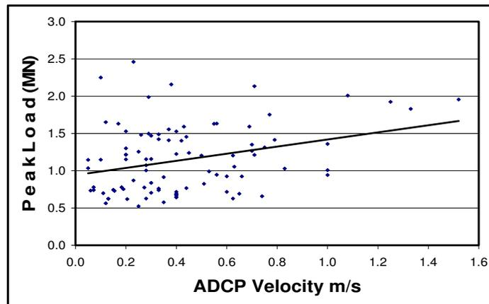
Figure 2a. ADCP Velocity Vs Peak Load for Keel Width Range of  $W_k < 20m$
