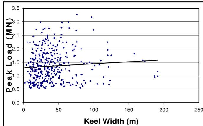
Figure 5b. Keel Width Vs Load for Keel Depth Range  $H_k < 11\text{m}$
