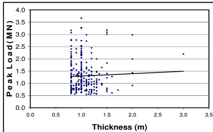
Figure 4a. Consolidated Layer Thickness Vs Load for a Range of  $H_c > 0.8m$
