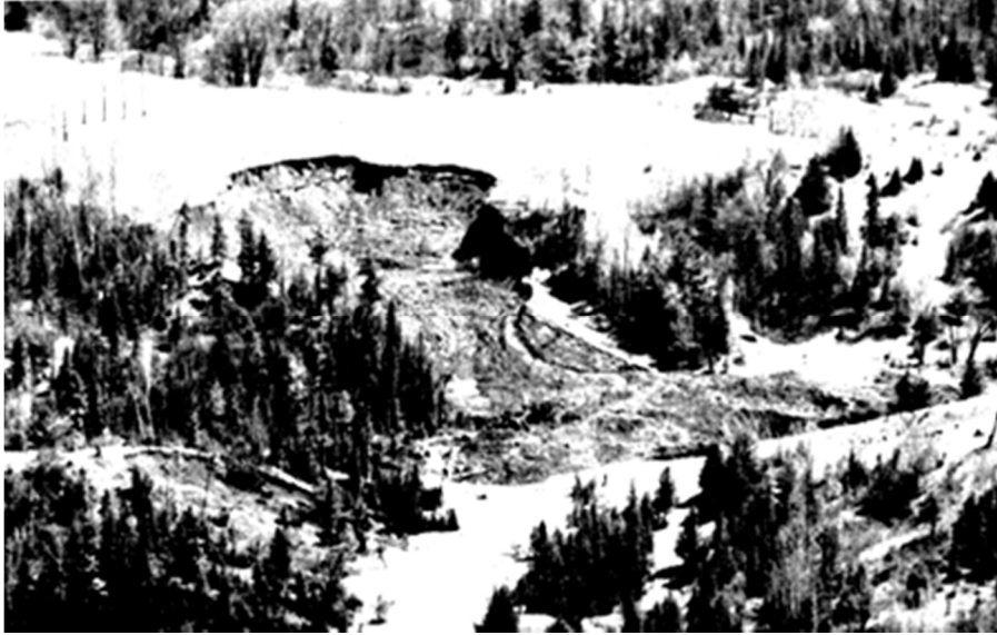
Figure 3. Landslides on Breckenridge Creek. (a) View of two small landslides that occurred in spring of 1969. (b) Aerial view of earthflow involving 30 000 cubic yards of clay that occurred on opposite bank in April 1963.
