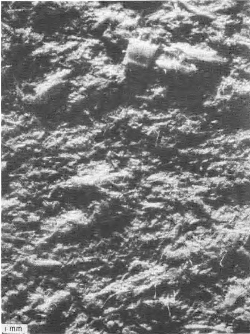
FIG. 5—Top surface of dry organic felt.
