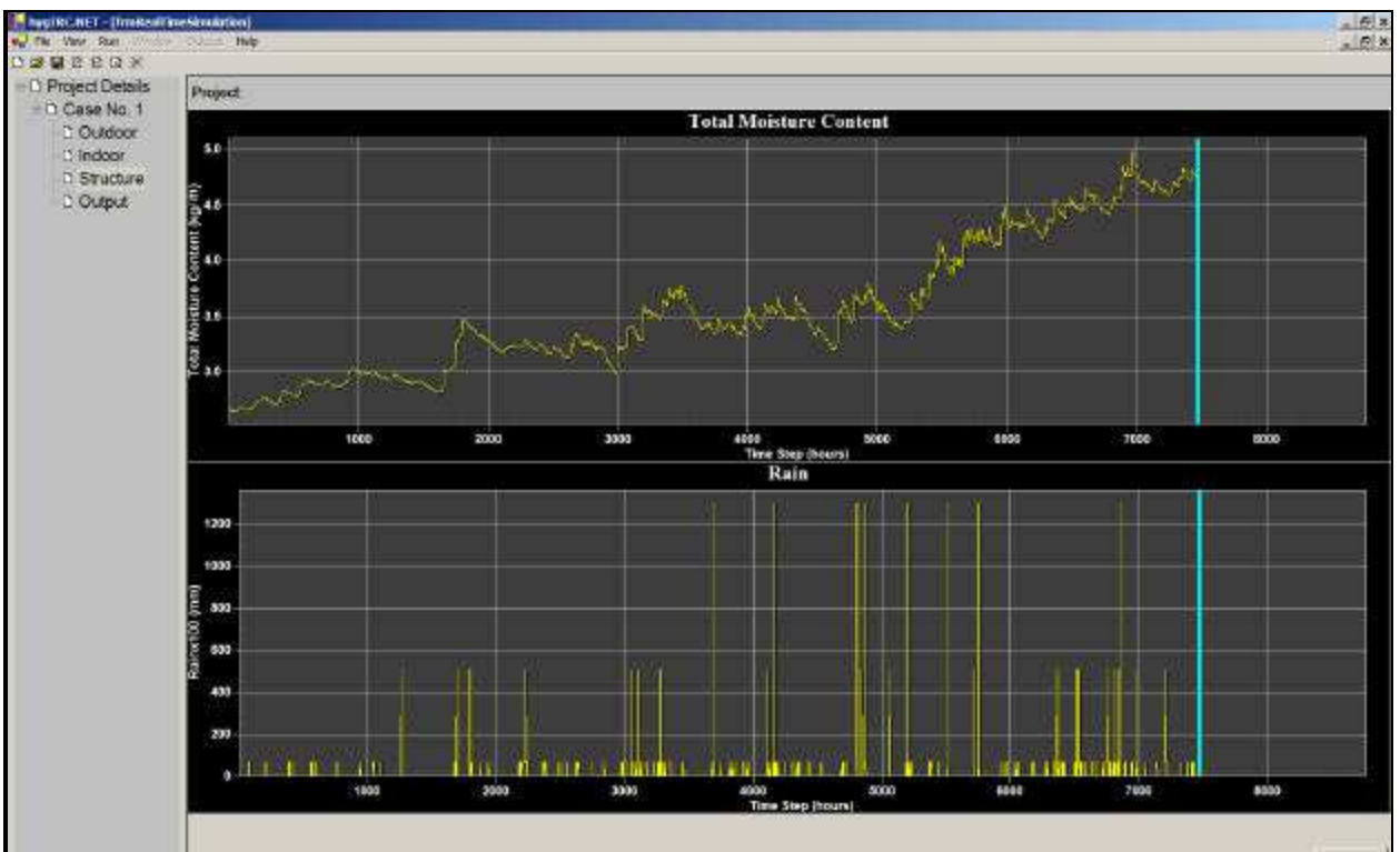
Figure 8. The screen shot shows the runtime operation of 1-D hygroIRC. The real time history of the total moisture content for all the wall layers is shown here along with the real time history of rain events derived from the weather file.
