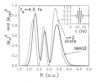
FIG. 2.  $|\Psi_{in}(R)|^2$  for the v = 2 vibrational state of  ${\rm H_2}^+$  plotted together with the simulated Coulomb explosion imaged  $|\Psi_{\rm CEI}(R)|^2$ . For this calculation the peak laser intensity was  $4 \times 10^{15}$  W/cm<sup>2</sup> and the time dependent electric field for the 4.5 fs full width at half maximum pulse is shown in the inset.
