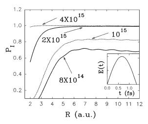
FIG. 1. Ionization probability for  $H_2^+$  in one-half period of 800 nm light plotted as a function of the internuclear separation for different peak laser fields. The fields are labeled by their corresponding laser intensity in W/cm<sup>2</sup>. The time dependent field of the  $\frac{1}{2}$ -period sine wave pulse is shown in the insert.
