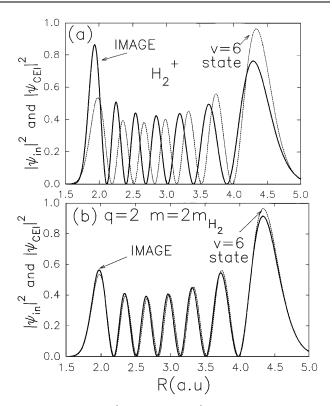
FIG. 4. (a)  $|\Psi_{in}(R)|^2$  and  $|\Psi_{CEI}(R)|^2$  obtained by an artificial Coulomb explosion where the ground state wave function is placed on the Coulomb repulsion curve. Note the similarity with Fig. 3(b). (b) When Coulomb explosion approximation is tested for higher mass and charge nuclei, the quality of reconstruction is greatly improved.
