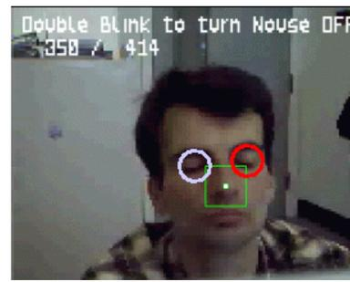
Fig. 6. Using double-blink to switch *Nouse* on/off.
