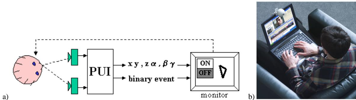
**Fig. 1.** Face-operated perceptual user interface: the system diagram (a) and the system at work (b). The photo picture shows a user at the moment of selecting a “Yes” button in a pop-up “Continue? Yes || No || Cancel” window, which is performed hands-free by using nose and double blinking.
