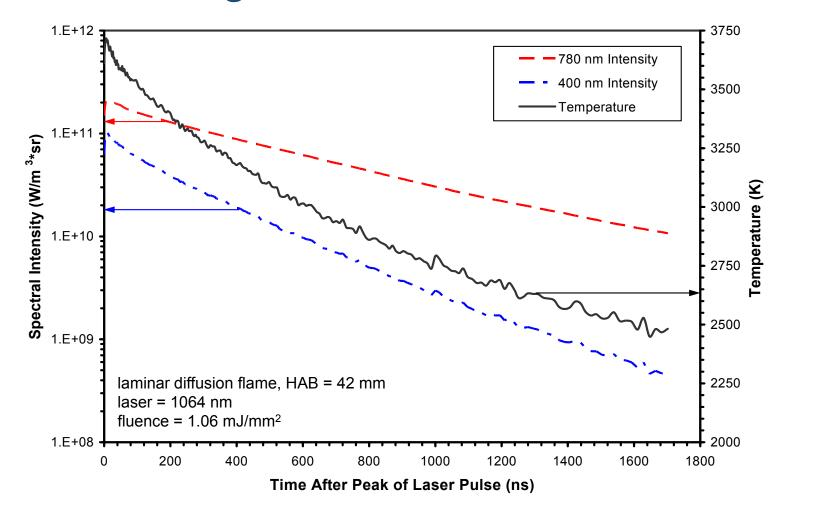
Laser-induced Incandescence (LII) for the Measurement of Atmospheric Black Carbon RC CRC 16 © Government of Canada
