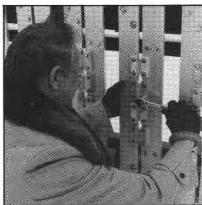
Figure 2. Specimens are bolted to rack.
