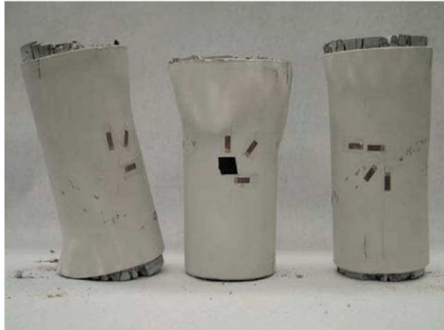
Figure 8: Failed concrete cylinders retrofitted with thermoplastic wrap (Uddin et al., 2008)
