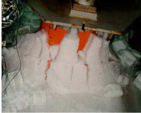
Figure 2. Photograph showing a typical ice interaction with the 45° cone: ice thickness equal to 115 mm and ice velocity equal to 0.01 m/s.
