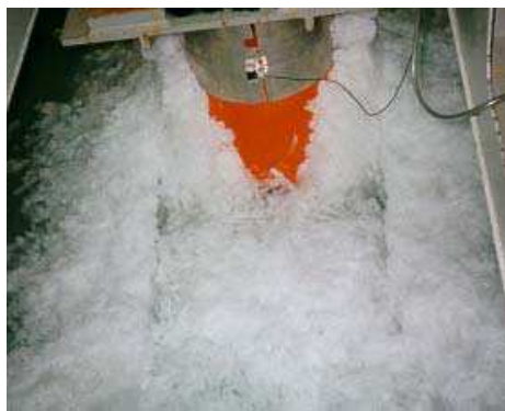
Figure 7. Photograph showing small columnar ice chips left at the wake of the 60° cone tested at high speed (ice velocity of 0.25 m/s)
