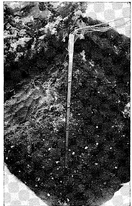
Fig. 2. Thermocouples located in test pit in clay; Ottawa, Ont.
