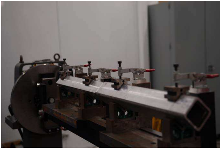
Figure 2: Experimental setup for tube welding.
