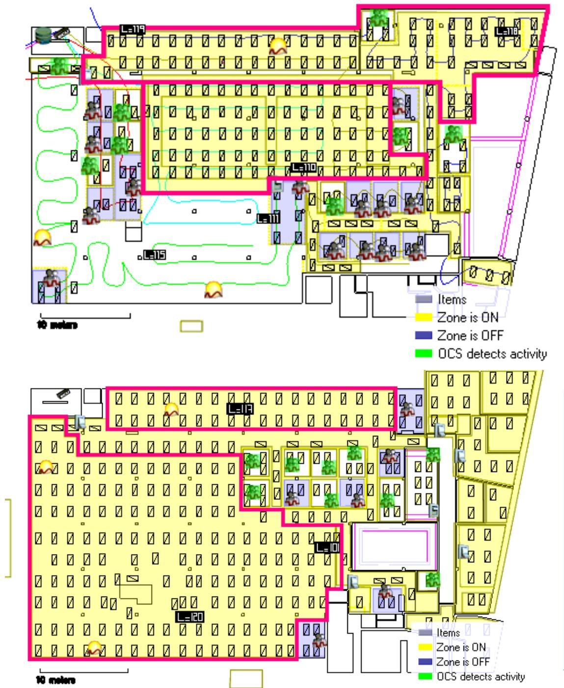
Figure 1. Floor and reflected ceiling plan of 1<sup>st</sup> (upper) and 2<sup>nd</sup> (lower) floors of the office building. The pink outlines show the four lighting zones that were independently controlled during the study. The yellow “sun-like” symbols indicate locations of photosensors, which were disabled on DR event days. Black boxes with text beginning “L=” indicate locations of illuminance loggers.
