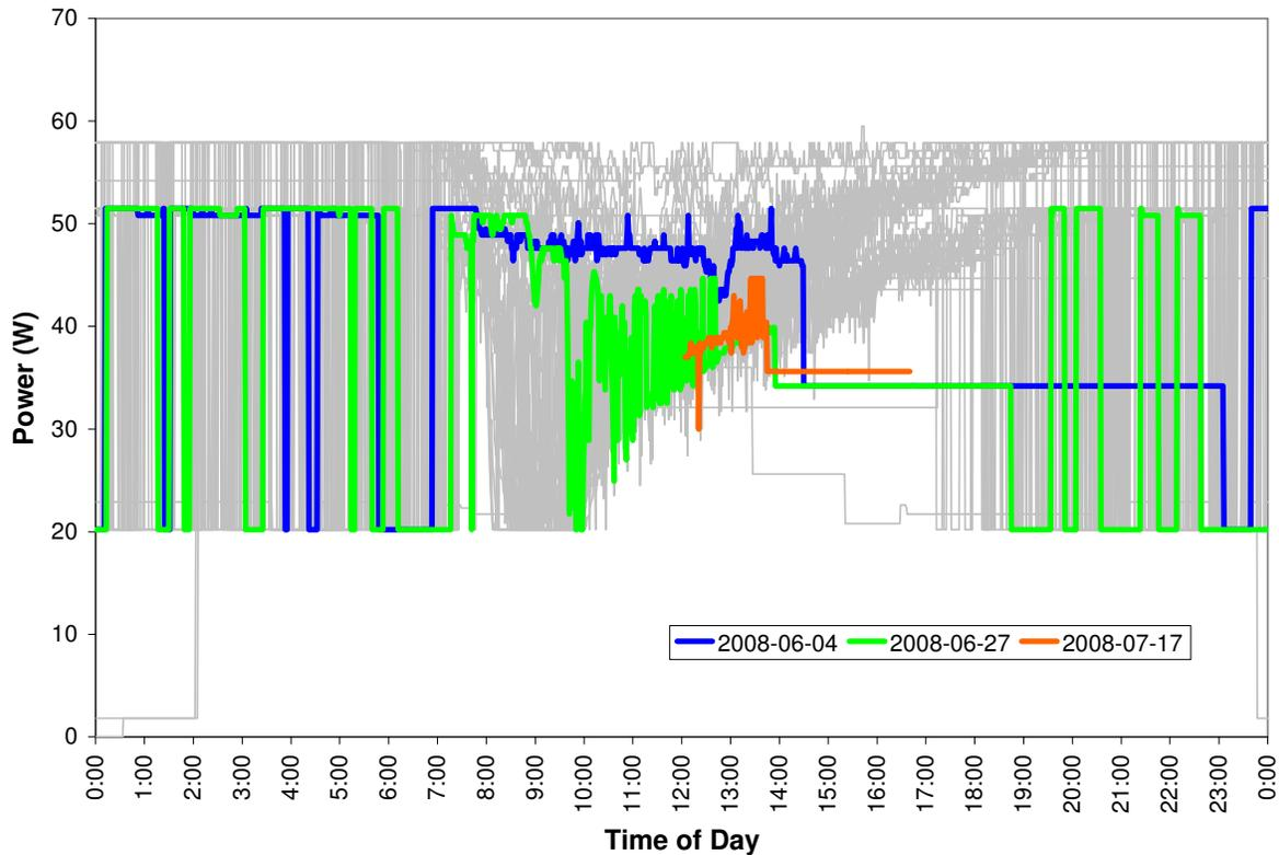
Figure 14. Calculated minute-by-minute lighting power for a single corridor ballast at the campus site, connected to a photosensor, for all normal weekdays (excluding public holidays). Non-DR days are shown in grey, DR days are shown by individually-coloured, thick lines. Periods of missing data appear as obvious gaps in the trace.
