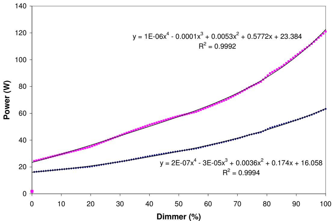
Figure 10. Dimmer/power curve fit to manufacturer's data for the college site; lower curve for 28W lamps, upper curve for 54W HO lamps. Note, the power drawn when the dimmer setting was zero was not continuous with these curves.
