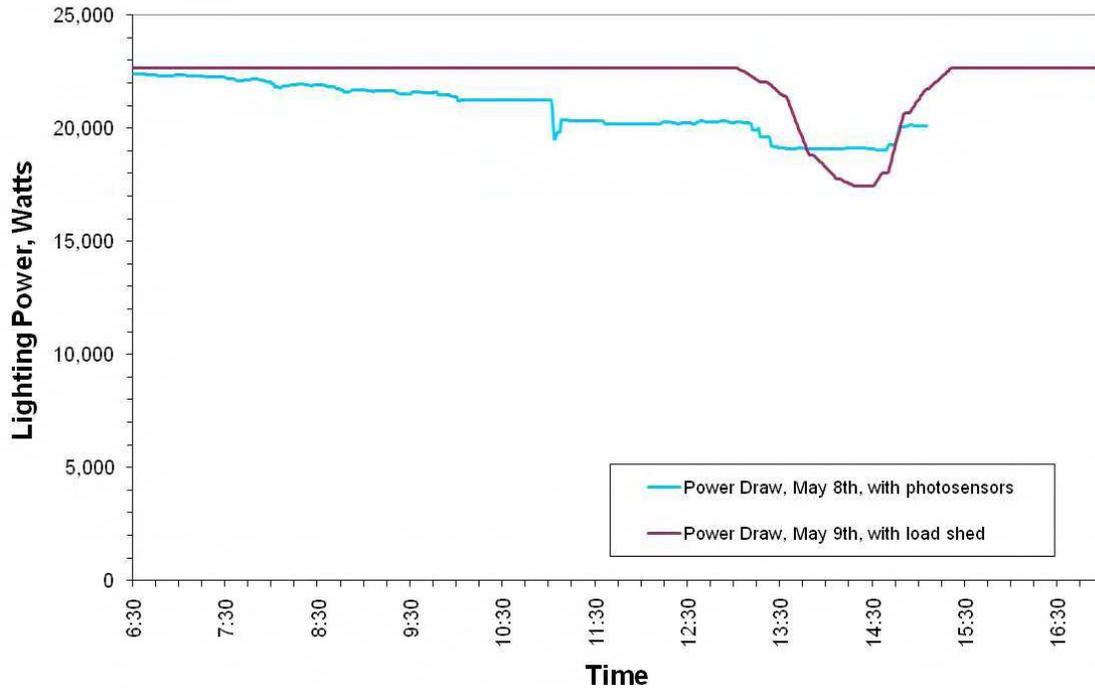
Figure 13. Derived power data at the office site for all study zones combined, for a non-DR day with photosensors active, and for the following DR day with photosensors disabled.
