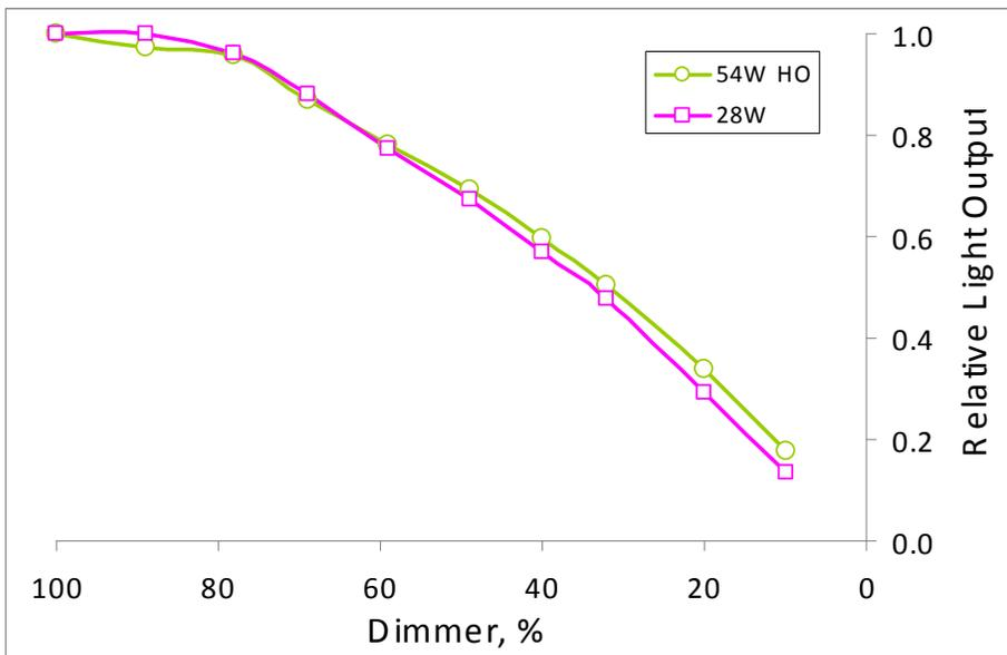
Figure 7. Dimming vs. relative light output curves, as measured at representative locations at the two sites. The upper chart shows data from each floor on the office site, measured under the same luminaire type. The lower chart shows data from the college campus, measured in an office with 54 W HO lamps only, and a classroom with 28 W lamps only.
