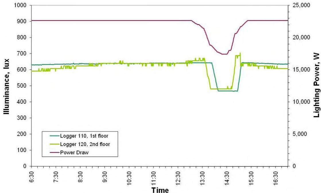
Figure 9(a). Derived power data for all study zones combined, and two example interior illuminance measurements, for the DR trial at the office building on May 9<sup>th</sup>.
