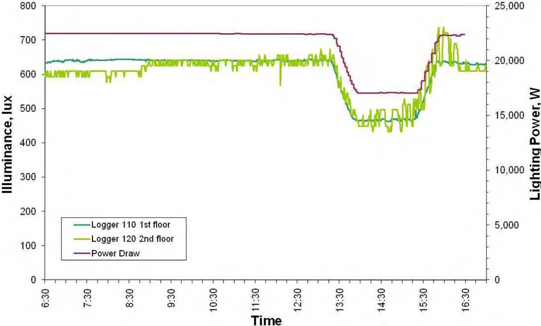
Figure 9(b). Derived power data for all study zones combined, and two example interior illuminance measurements, for the DR trial at the office building on May 23<sup>rd</sup>.
